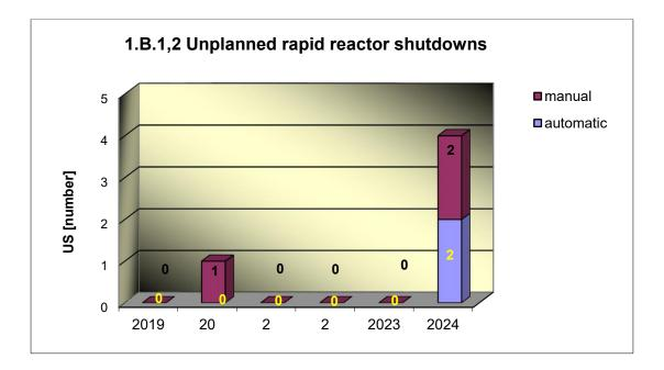
Graph 1.B.1,2a compares the number of unplanned rapid reactor shutdowns (US), including manual shutdowns, by unit.
