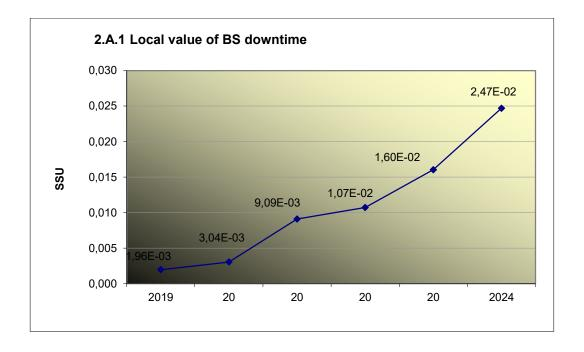
The non-operability of individual BS (SSU<sub>S</sub>) – graphs 2.A.1.a - g - is defined as the ratio of the total non-operability time of the evaluated BS to the total time during which its operability was required. These combined graphs also show the ratio of the non-operational time of a given BS to the "general" BS of the site.
