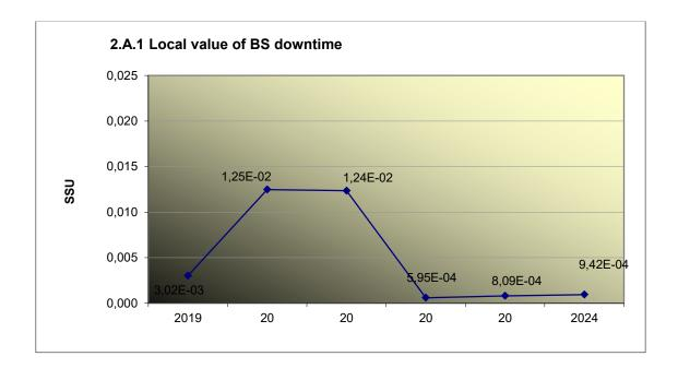
The non-operability of individual BS (SSU $_{\rm S}$ ) - graphs 2.A.1.a – g, is defined as the ratio of the total non-operability time of the evaluated BS to the total time during which its operability was required. These combined graphs also show the ratio of the non-operational time of a given BS to the "general" BS of the site.
