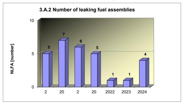
Graph 3.A.2a shows the number of leaking fuel assemblies by unit.
