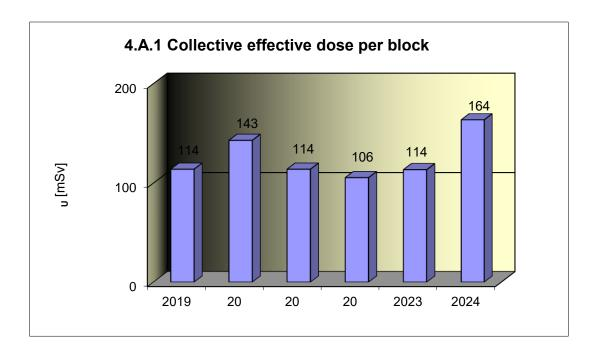
Graph 4.A.2 shows the collective effective dose, which is given by the total external whole-body dose received by radiation workers at NPPs and suppliers during the monitored period.
