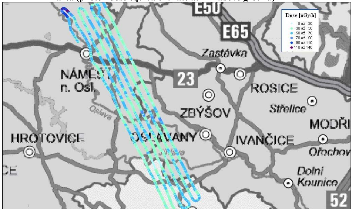
Figure No.6 Air monitoring results within Náměšť nad Oslavou – Moravský Krumlov area (photon dose equivalent rate at 1 m above ground)
