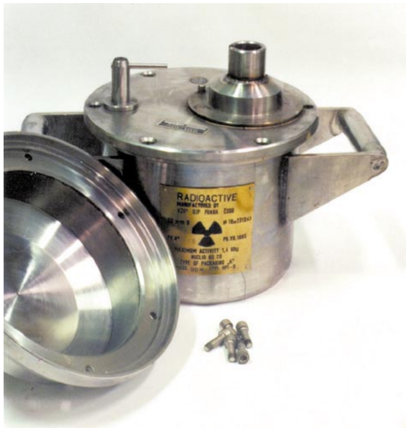
Figure 6.28 The HPT-6 transport container, class A, uranium shield, diameter of 25 cm, height of 27 cm, weight of 80 kg. Intended for transport of the maximum 1.4 GBq of ^{60}\text{Co} , but also for ^{137}\text{Cs} and the other nuclides
