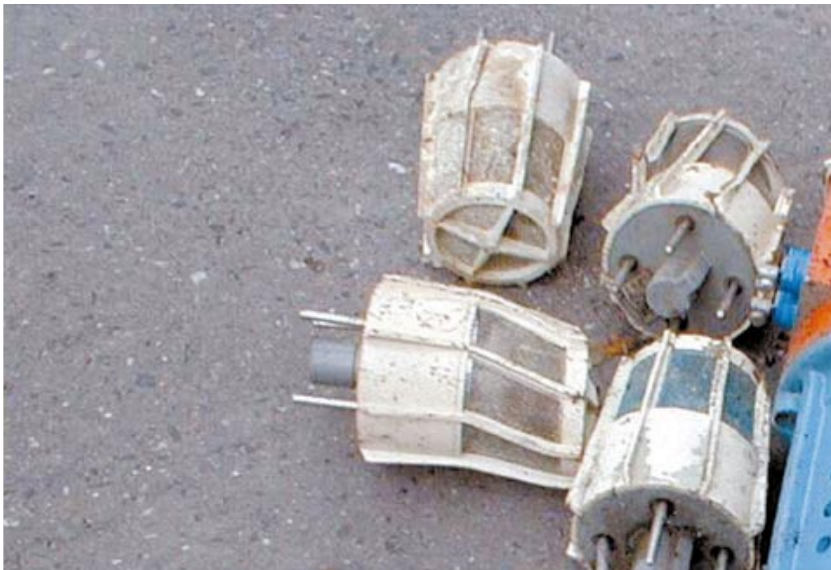
Figure 7.8 The fire detectors with ^{226}\text{Ra} or ^{241}\text{Am} that were found in municipal waste. Activity of ^{226}\text{Ra} ~ 50 kBq, activity of ^{241}\text{Am} ~ 1MBq, dose rate in contact from 0.1 to 3 \mu\text{Gy/hr} . The photograph supplied by SÚRO
