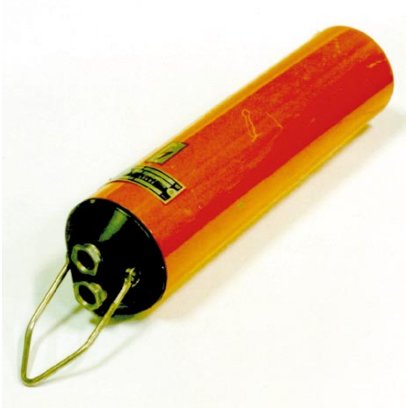
Figure 3.10 The MKD 103 level indicator probe. The probe itself does not contain any source, however any following source produced by the former Tesla Liberec may be assembled inside the probe: MDG 300, MDG 301 or MDG 201
