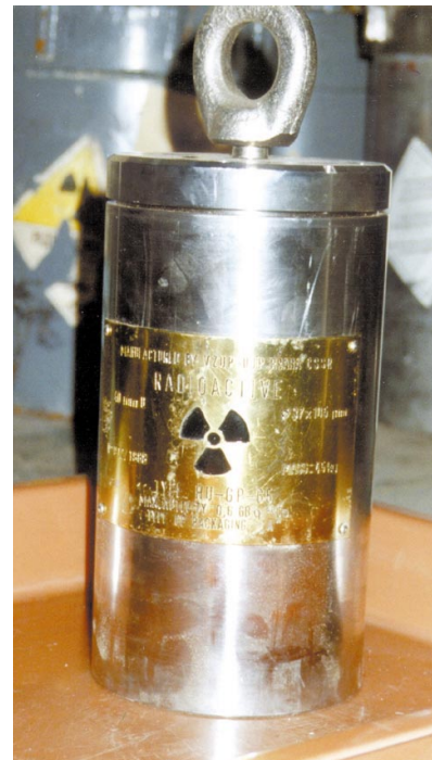
Figure 6.2 The HU-GP-65 transport container, the new version with a lug on the top
