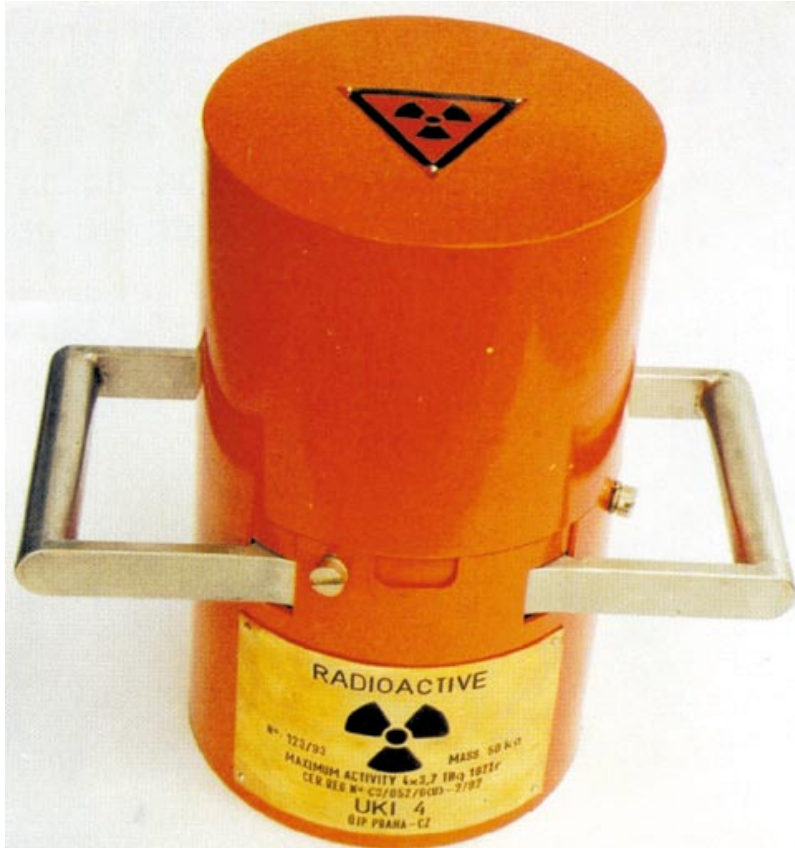
Figure 6.18 The UKI-4-135 type transport container, class B, in a transport package. Uranium shield, 17cm \times 28cm, and weight of 50 kg. Maximum activity of 4x3.7 TBq of 192Ir. From the ŠKODA – ÚJP, Praha, a.s. company documentation
