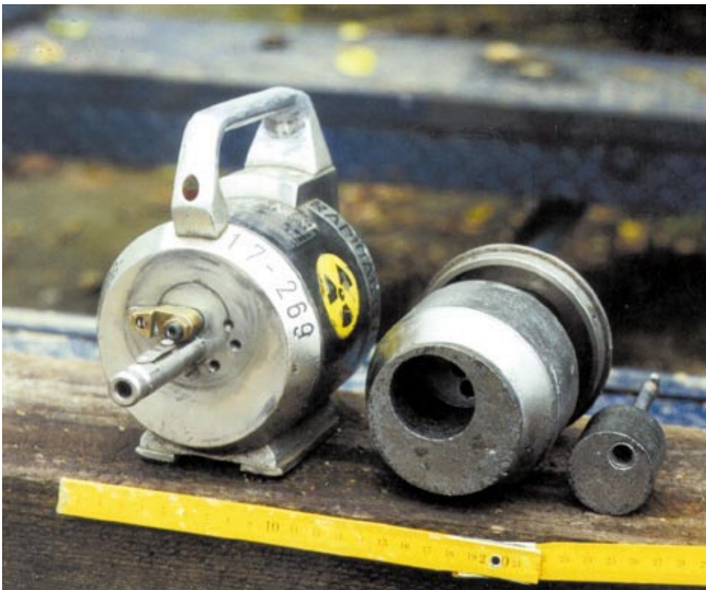
Figure 4.15 The dismantled Gammamat TIF. The other view
