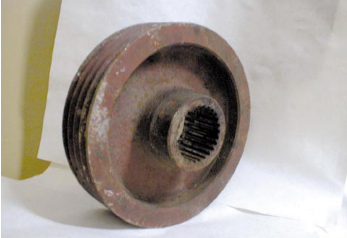
Figure 7.11 The metallurgical products that are contaminated by ^{60}\text{Co} from randomly melted sources. Their activities are in a range from tens of kBq/kg up to tens of MBq/kg. Dose rates in contact from 1 to 100 \mu\text{Gy/hr} . Pulley. The photograph supplied by SÚRO
