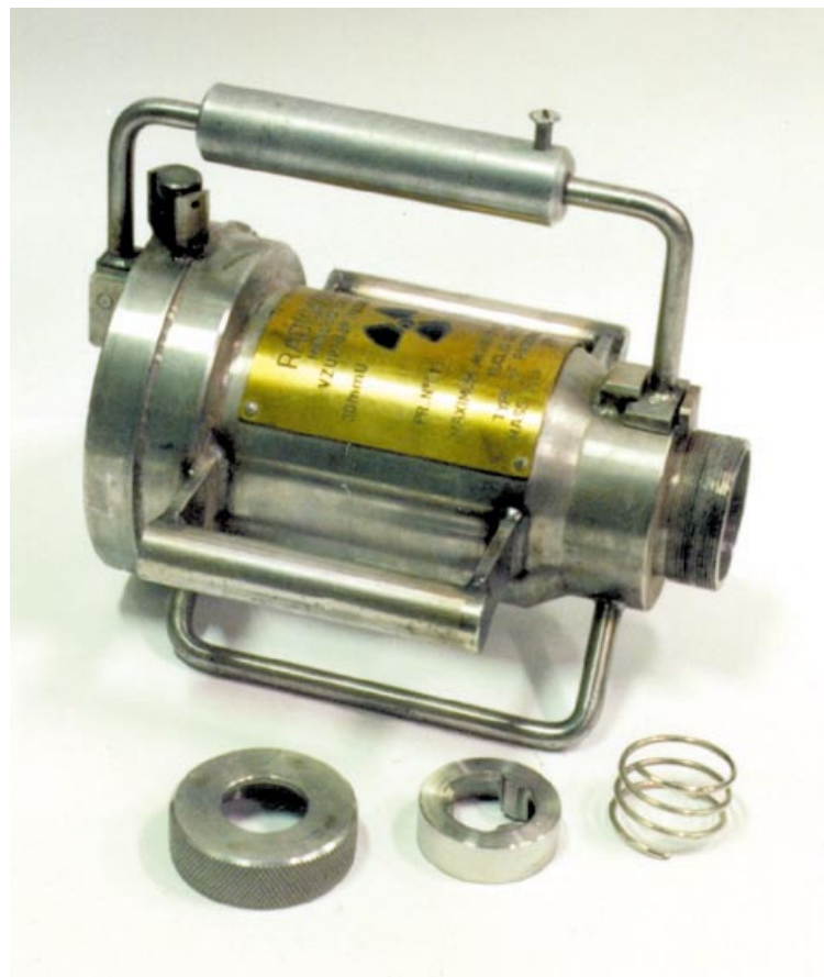
Figure 6.31 The HPT-1 „temporary storage” container, class A, 52 mm uranium shield, cylinder diameter of 13 cm, length of 24 cm, weight of 39 kg. Used for temporarily storing max. 3.2 GBq of ^{60}\text{Co}
