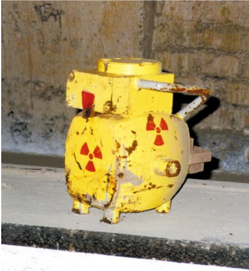
Figure 3.33 The Polish PrI-20 operational container, Pb shield, and its weight of 48 kg
