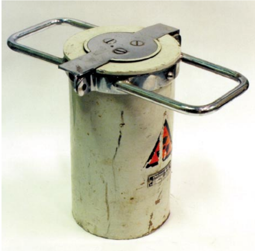
Figure 5.5 The Chirana 392 type lead transport container, produced about 1970. Its height is 26 cm, diameter of 14 cm and weight of 42 kg
