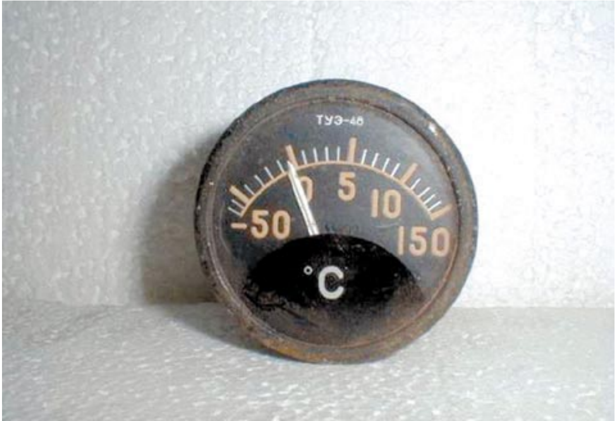
Figure 7.5 The military device coated with a ^{226}\text{Ra} luminescent paint that was found in metal scrap. Activity from 50 to 500 kBq, dose rate in contact from 1 to 10 \mu\text{Gy/hr} . The photograph supplied by SÚRO
