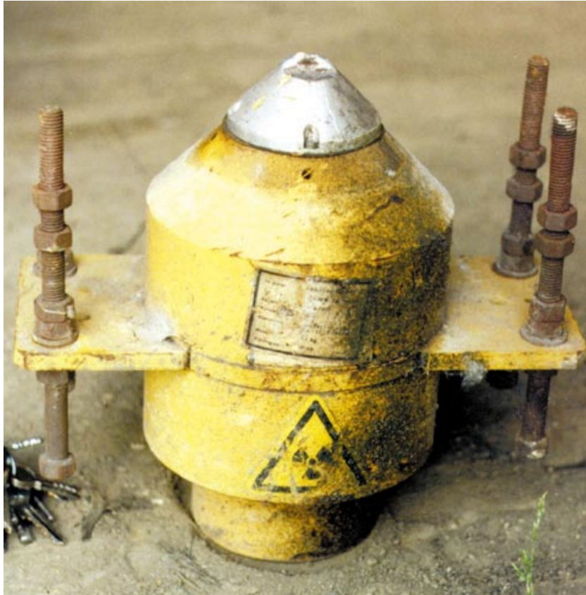
Figure 3.22 The operational container for the ash-gauge produced in the former East Germany. The container with a conical shield - the source is in the operating state. Size of about 25 cm, weight of 44 kg
