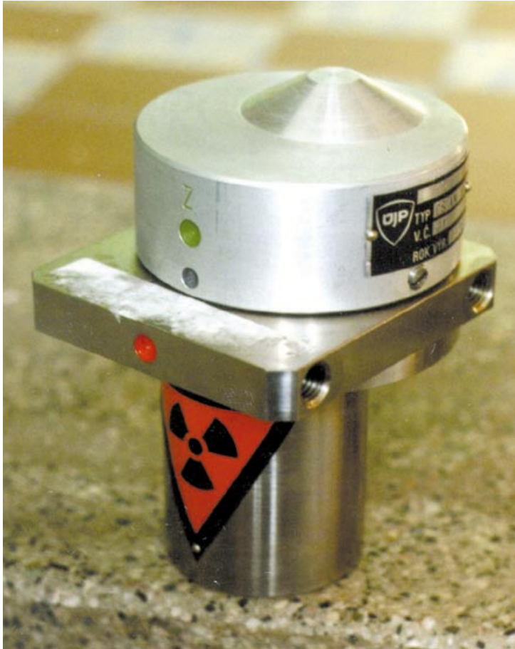
Figure 3.18 The CsAm 16/II operational container, used in the GE 1100 S gamma ash-gauge. The gauges contain 2 different sources: one alpha source and one gamma source, in this case ^{241}\text{Am} 12 GBq and ^{137}\text{Cs} 0.62 GBq. Depleted uranium shield. Height of about 16 cm. Product of ŠKODA - ÚJP, Praha, a.s.
