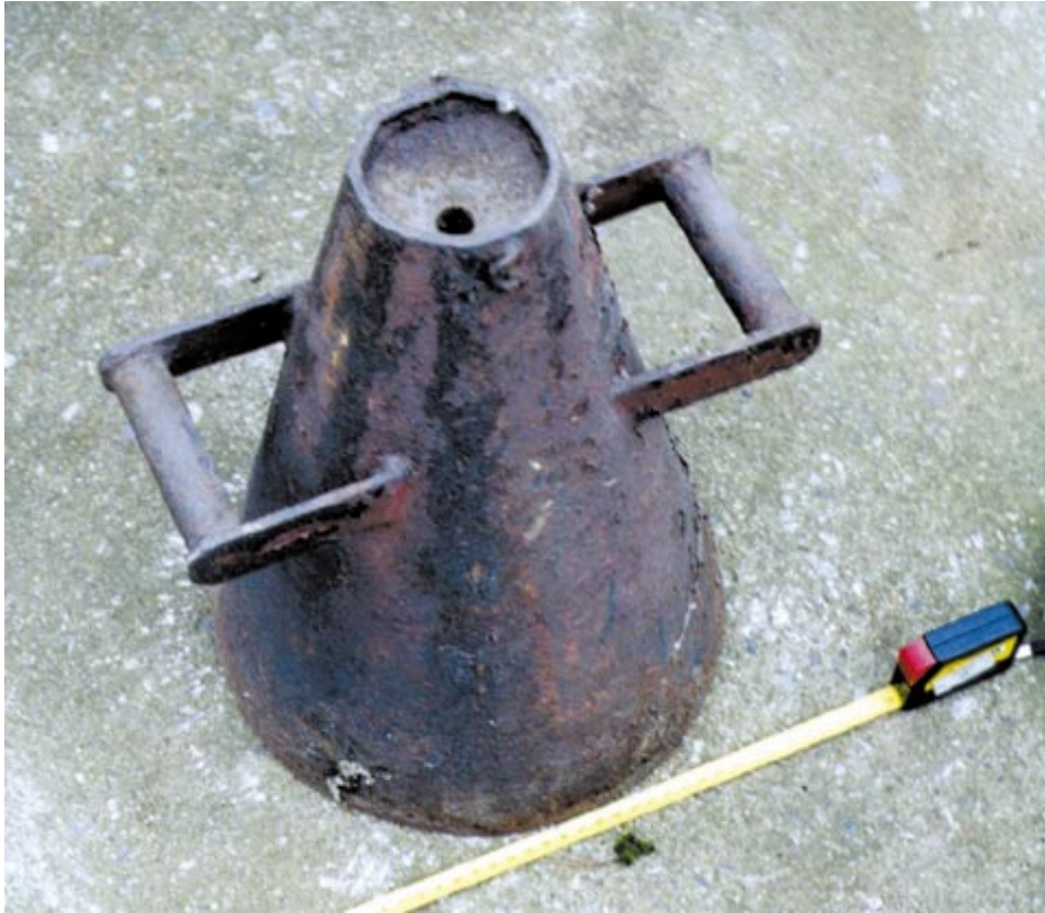
Figure 4.26 A conical container that was used perhaps for transport, however due to its weight of about 70 kg was used as a temporary shield for storing a bar with flaw detector source (see for example in Fig. no 4.17). The diameter of the bottom is 27 cm, a height of 38 cm. Steel jacket and lead shield
