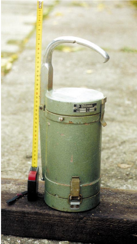
Figure 5.3 The Chirana M 6102 transport container. This container was used for medical source transport including liquid source and water sample transport from the primary circuit of nuclear power plants. Lead shield, its weight of 31 kg. The container is typical with its separated bottom
