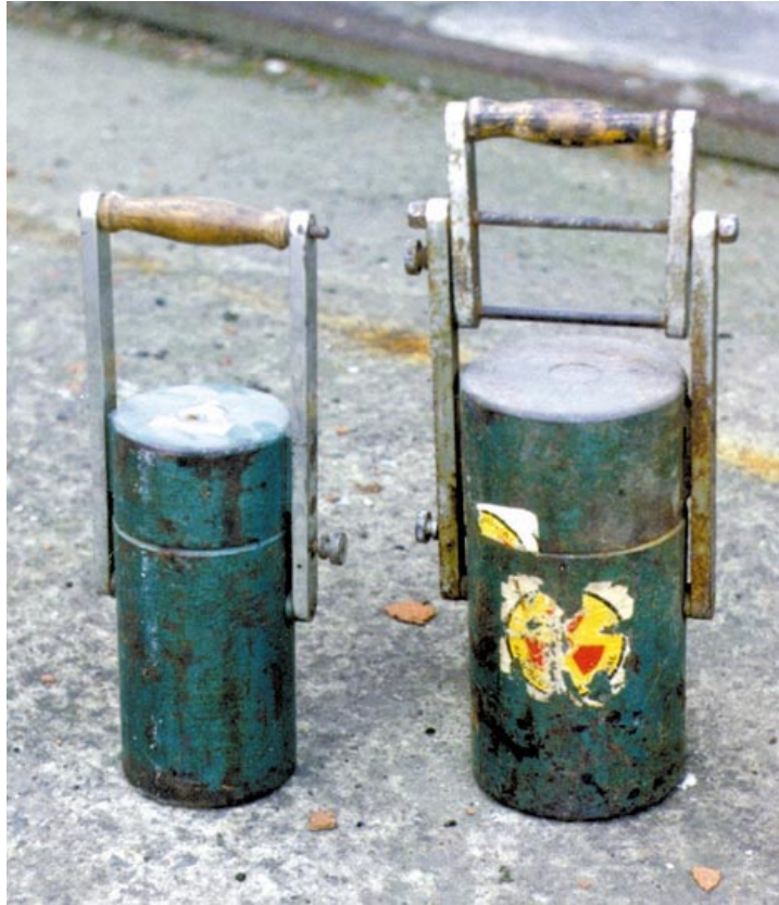
Figure 6.44 The OK-25 and OK-35 source lead transport containers. Height of about 30 cm, weight of 25 kg or 35 kg. Produced by ÚJP Praha
