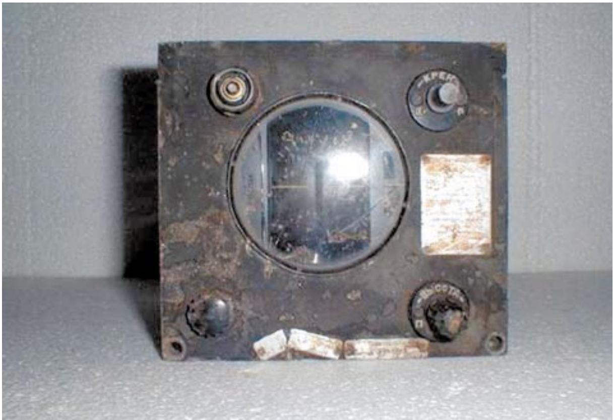
Figure 7.6 The other military device coated with a ^{226}\text{Ra} luminescent paint. The photograph supplied by SÚRO
