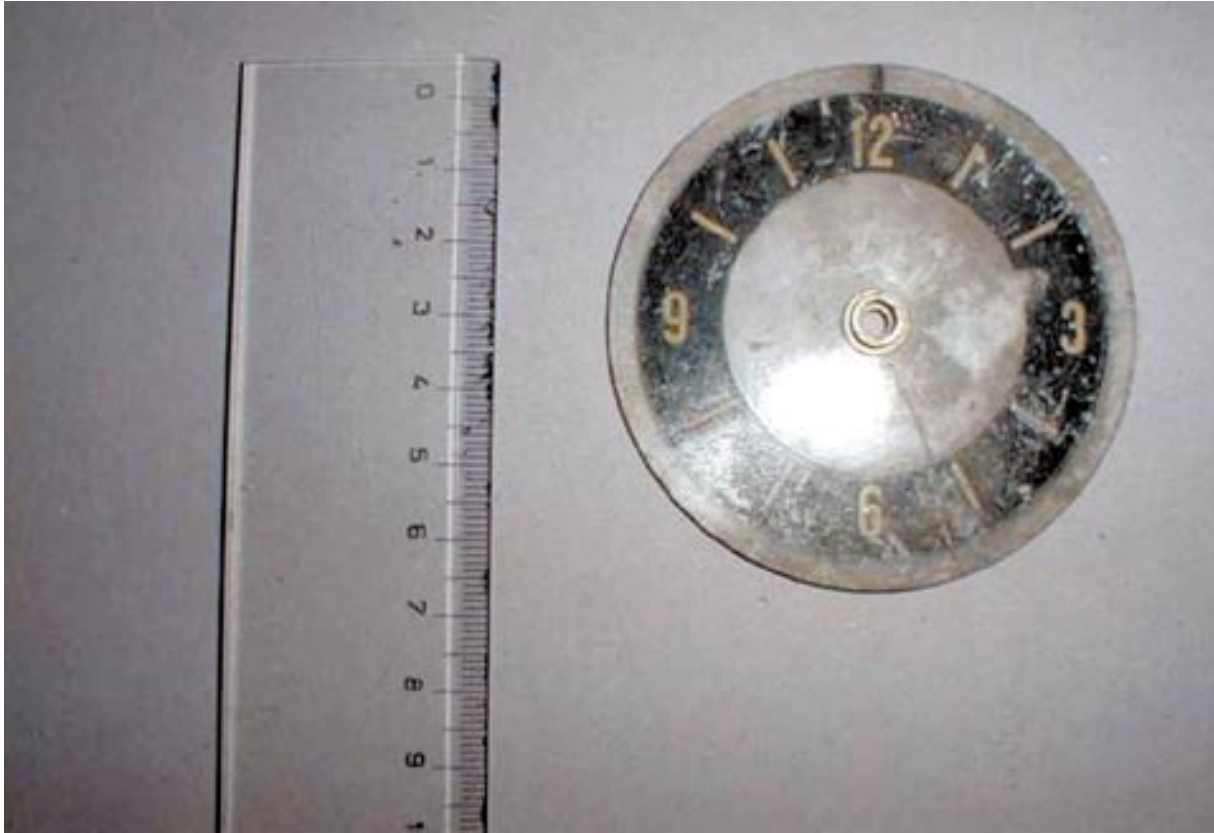
Figure 7.3 The semi-product of a clock dial coated with a ^{226}\text{Ra} and ^{90}\text{Sr} luminescent paint that was found in municipal waste. Activity in order of MBq, dose rate in contact from 100 to 300 \mu\text{Gy/hr} . The photograph supplied by SÚRO
