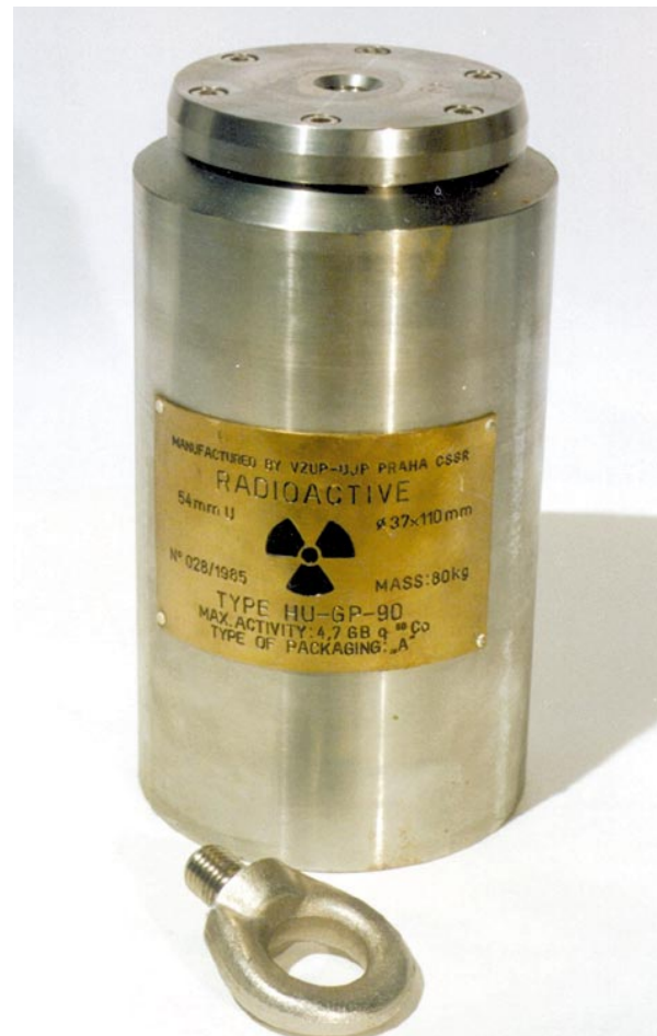
Figure 6.5 The HU-GP-90 transport container. This is the newest container of the HU-GP series. Dimensions of 15.6cm \bar{\iota} 35cm, weight of 80 kg. The container can contain different sources of activities up to units of GBq (for ^{60}\text{Co} ). The photograph from ŠKODA – ÚJP Praha, a.s.
