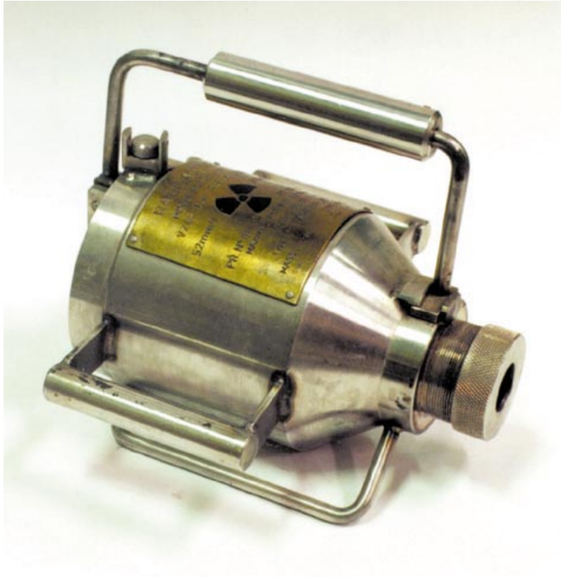
Figure 6.30 The HPT-1/L „temporary storage” container, class A, 30 mm uranium shield, dimensions of 18cm (cylinder diam. of 9cm) i 22 cm, weight of 18.5 kg. Max. 0.234 GBq of ^{60}\text{Co}
