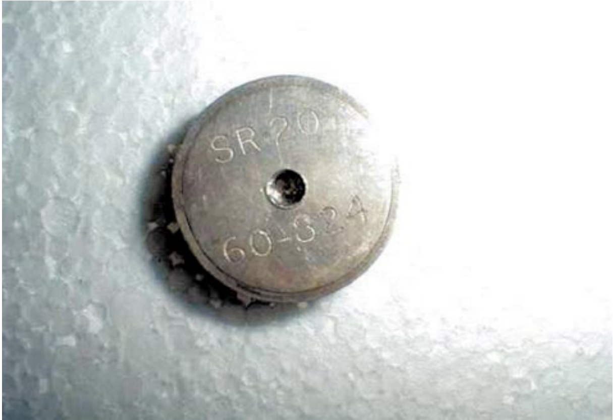
Figure 7.15 The ^{90}\text{Sr} source of the thickness gauge which was found in metal scrap. The original activity was 740 MBq, dose rate at a distance of 1 m is about 1 \mu\text{Gy/h} . The photograph supplied by SÚRO
