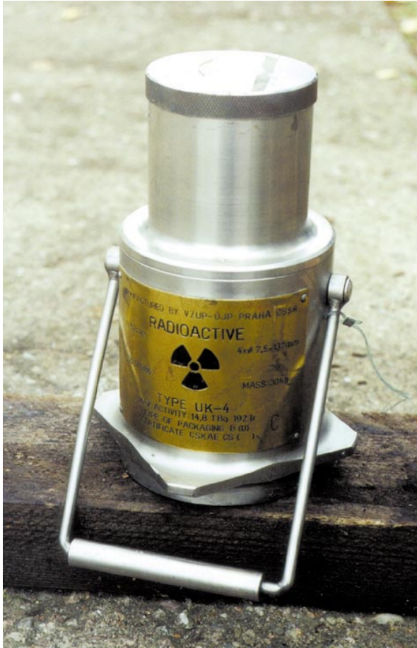
Figure 6.15 The UK-4 transport container. This is intended for transport of max. 14.8 TBq of ^{192}\text{Ir} (flaw detector sources). The height of 27 cm, 52 mm uranium shield, and its weight of 30 kg. The container is now banned and replaced by the UKI-4-135 type
