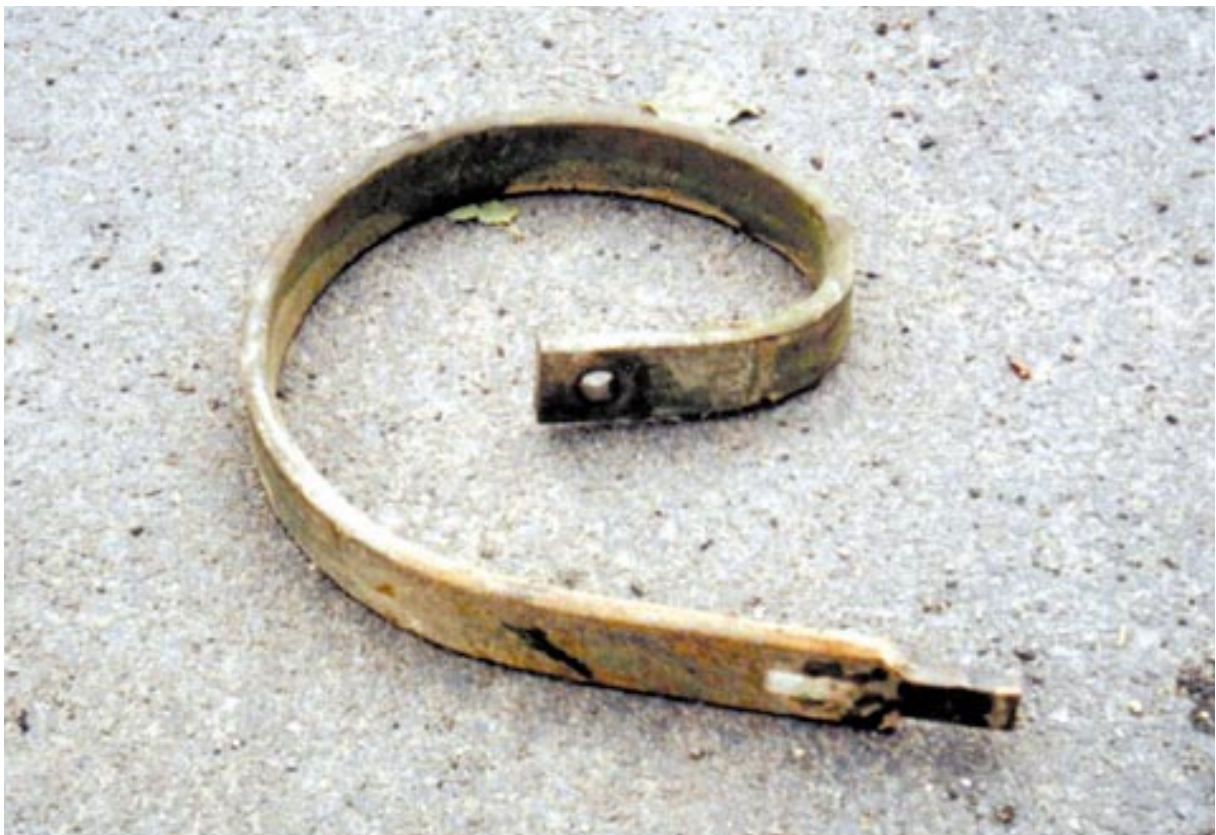
Figure 7.14 The elastic cultivator blade holder that is made in ^{60}\text{Co} contaminated heat. The specific activity in the year 2000 was about 2 \text{ MBq/kg} , dose rate in contact of about 500 \text{ } \mu\text{Gy/hr} . The photograph supplied by SÚJB
