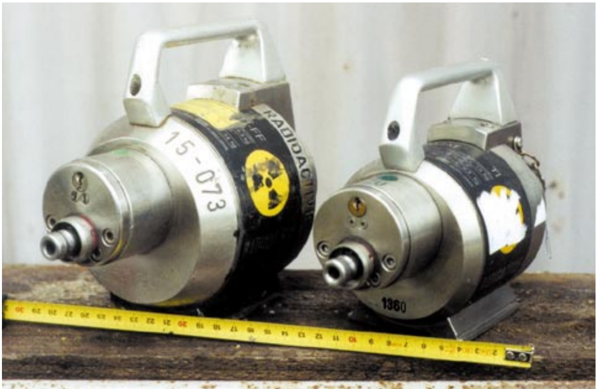
Figure 4.13 The flaw detectors that are used at present days: on the left: Gammamat TI-FF (18.5 kg, of this 14 kg depleted uranium, source max. 4.884 TBq of ^{192}\text{Ir} ), on the right, Gammamat TI (13 kg, 9.4 kg uranium, max 1.5 TBq of ^{192}\text{Ir} ). Produced by VKTA Rossendorf, Germany
