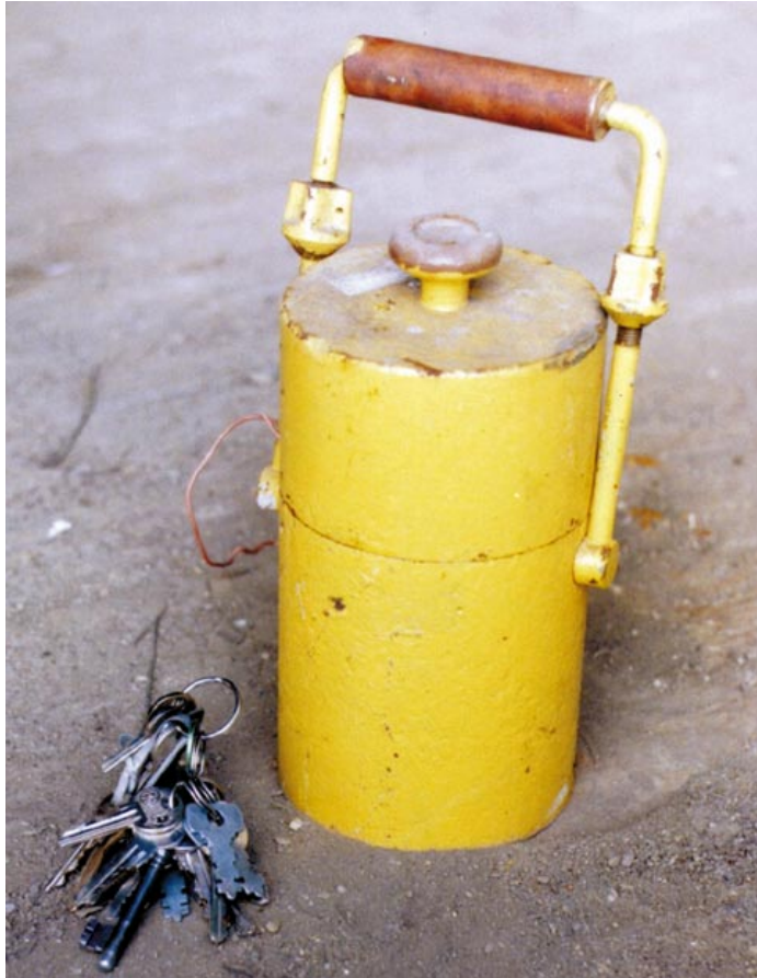
Figure 6.46 The old type of the transport container. Lead shield. Coating not original
