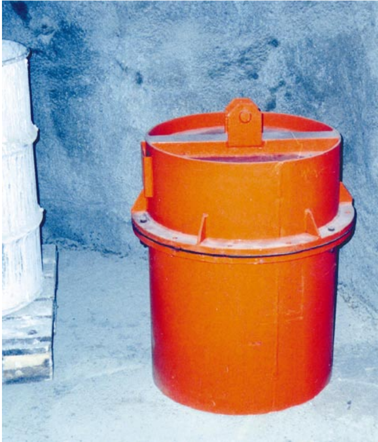
Figure 6.40 The transport package prototype for large containers. Diameter of about 35 cm
