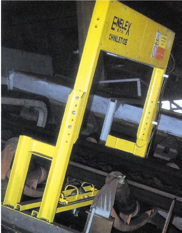
Figure 3.16 The GE 1100.S gamma ash-gauge, the general view on the equipment. The source is placed below the belt, the shield top is seen between two yellow "lugs" Produced by Enelex, Chvaletice, the Czech Republic. From the company documentation of Enelex, s.r.o. Chvaletice, the Czech Republic
