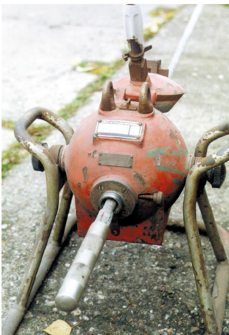
Figure 4.18 The OK 0.5 flaw detector – the rear view on the operational position with the ejected source
