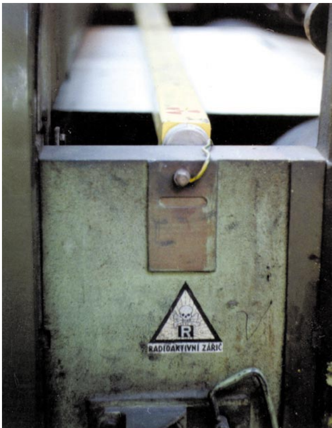
Figure 1.3 The electrostatic charge eliminator (the yellow bar above) on a rubber coating machine. The high-intensity alpha radiation eliminates electrostatic charge on the surface and it also reduces the danger of explosion due to thinner vapour
