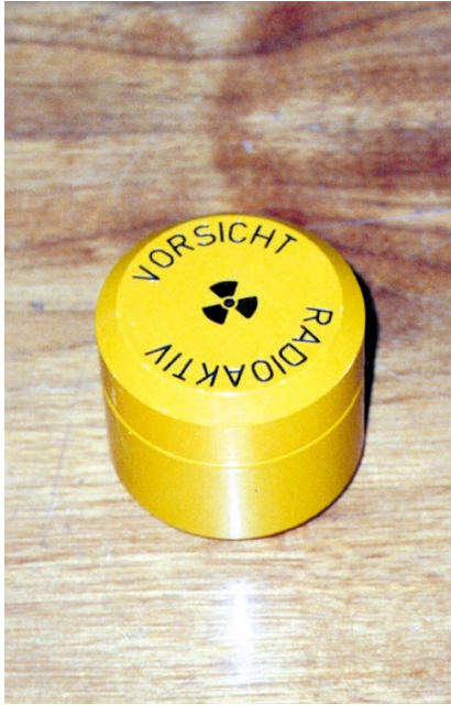
Figure 6.50 The FH 35 small container, made in Germany, dimensions of 6cm \bar{\bar{}} 6cm, weight of about 1.5 kg
