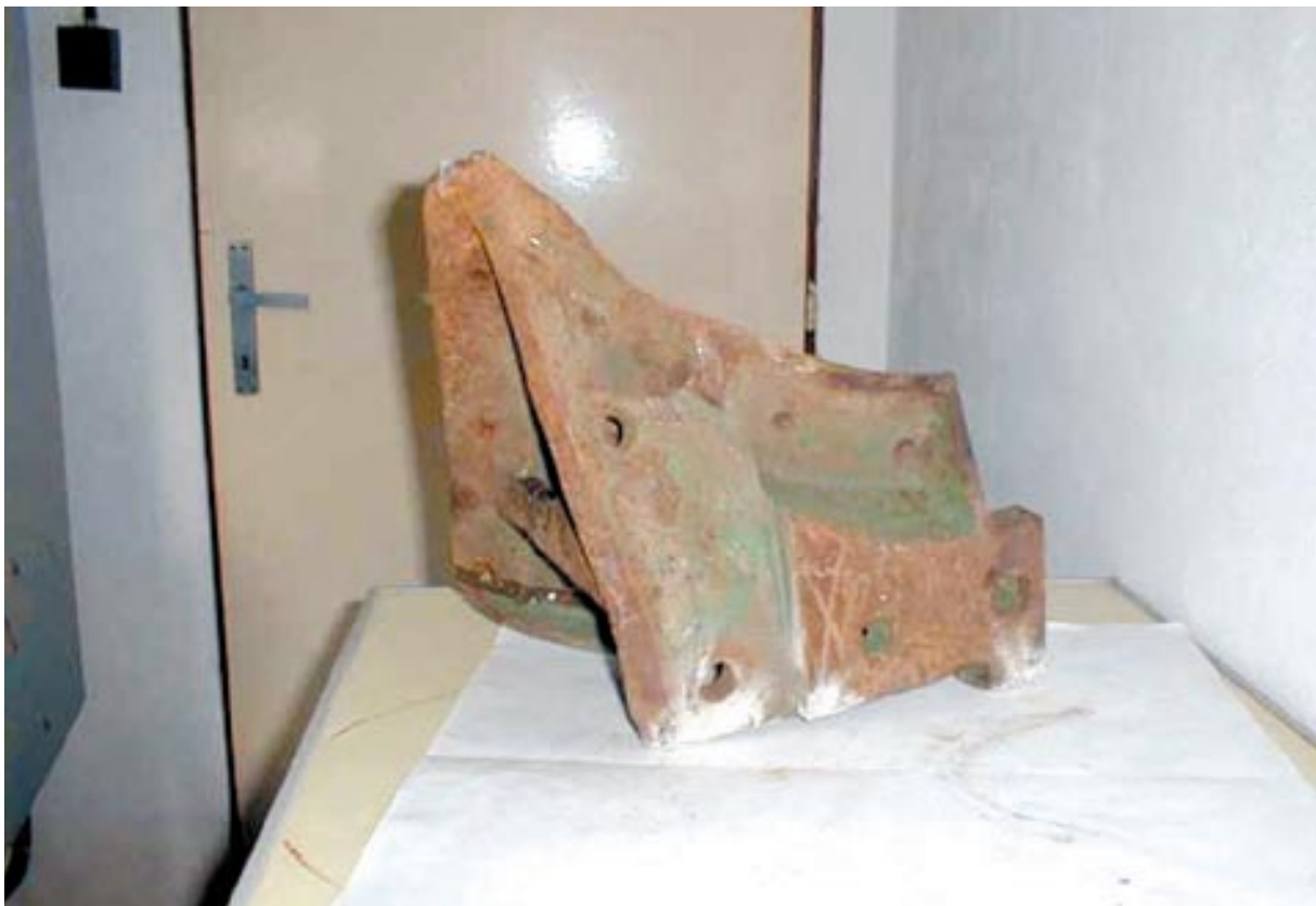
Figure 7.12 The metallurgical products that are contaminated by ^{60}\text{Co} from randomly melted sources. Their activities are in a range from tens of kBq/kg up to tens of MBq/kg. Dose rates in contact from 1 to 100 \mu\text{Gy/hr} . Blade. The photograph supplied by SÚRO
