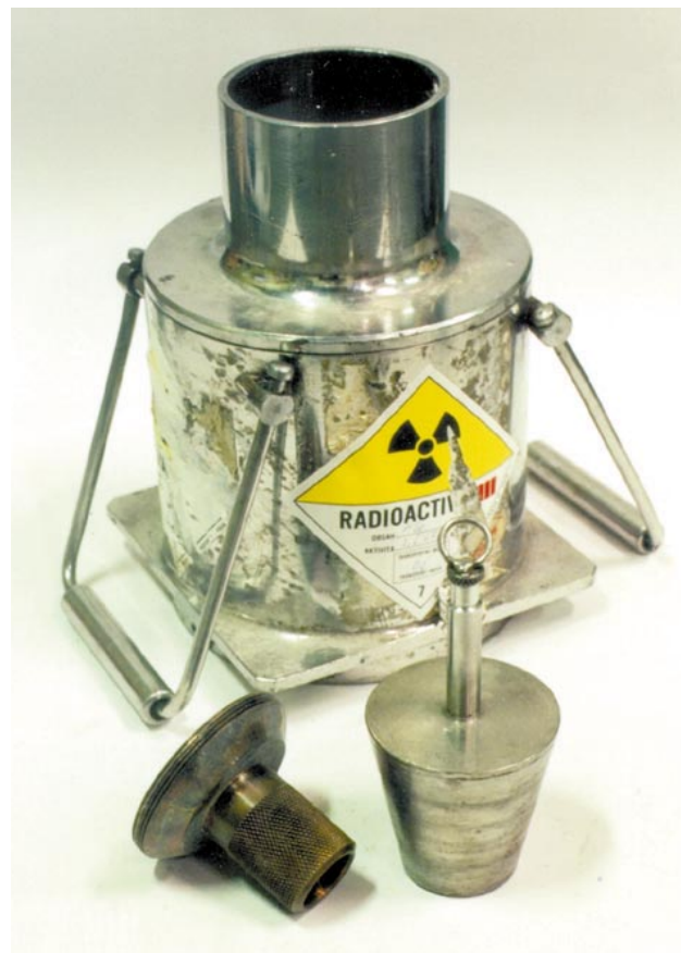
Figure 6.14 The open UK 8 transport container
