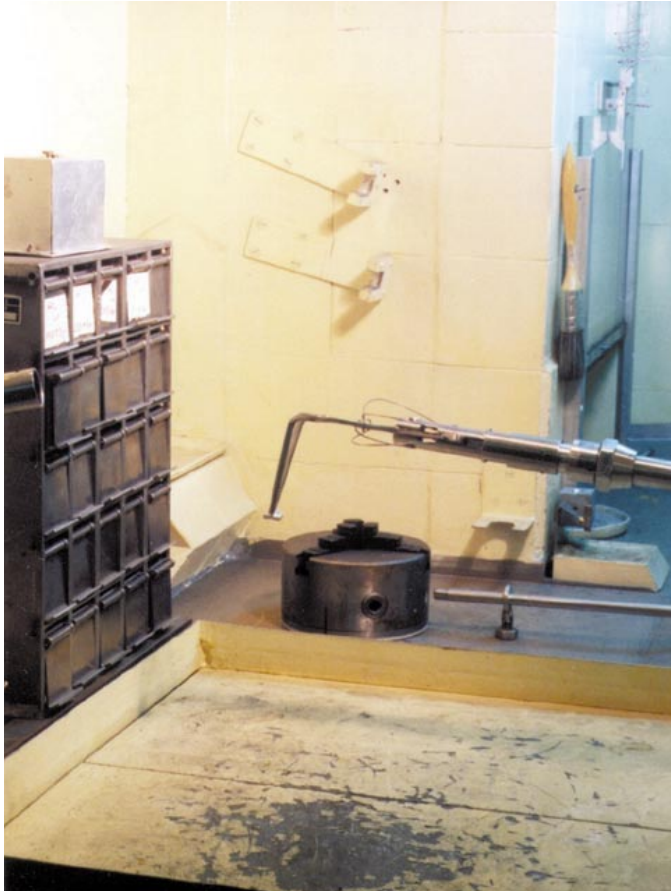
Figure 1.9 The interior of the semi-hot chamber. On the background, you can see the remote-controlled lathe head that is used for the source fixation
