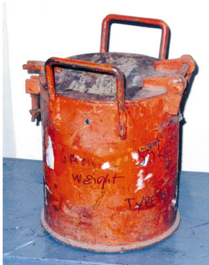
Figure 6.35 The transport cask for the Soviet container. Coating is not original. Dimensions of about 25cm \bar{\imath} 40 cm. Weight of 55 kg
