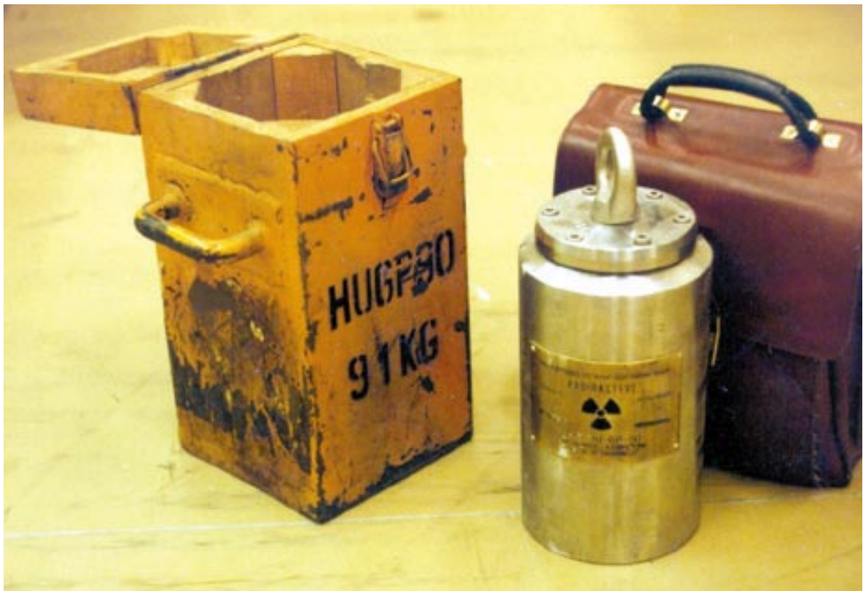
Figure 6.7 The HU-GP-90 container and its transport box
