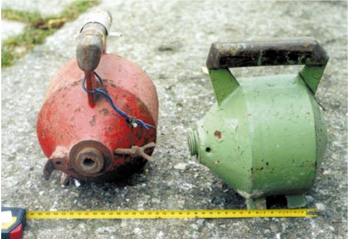
Figure 4.24 The old transport and operational containers for flaw detection. A bigger and heavier version of the "egg-shaped" containers (about 27 kg) is shown in Fig. 4.19 and 4.20. They were probably used only for transport because the internal channel is not straight-way
