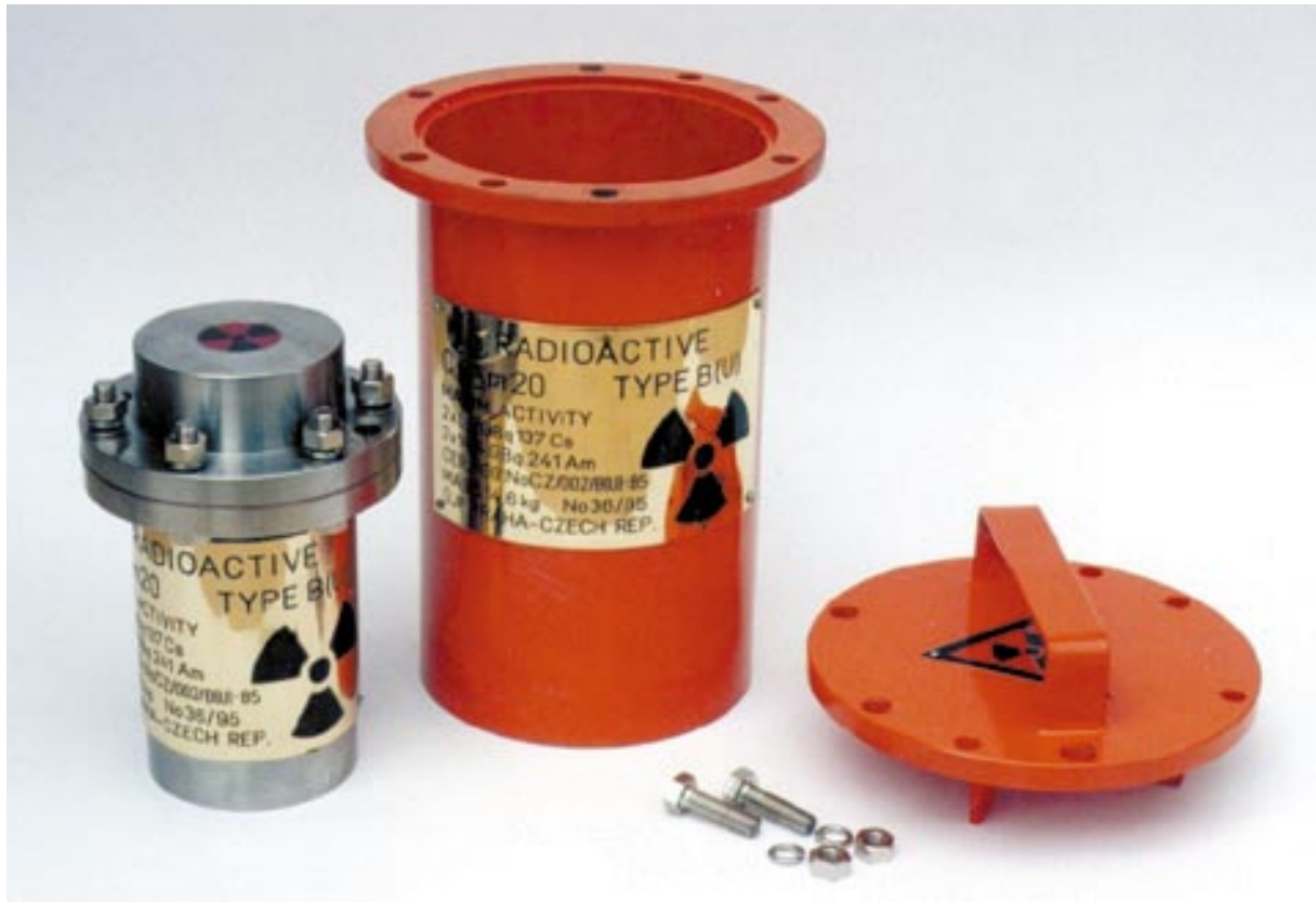
Figure 6.26 The CsAm20 type transport container, class B, with a transport package. Uranium shield, dimensions of 16cm \times 26cm. Weight of 14.6 kg. ÚJP Praha. From the ŠKODA – ÚJP, Praha, a.s. company documentation
