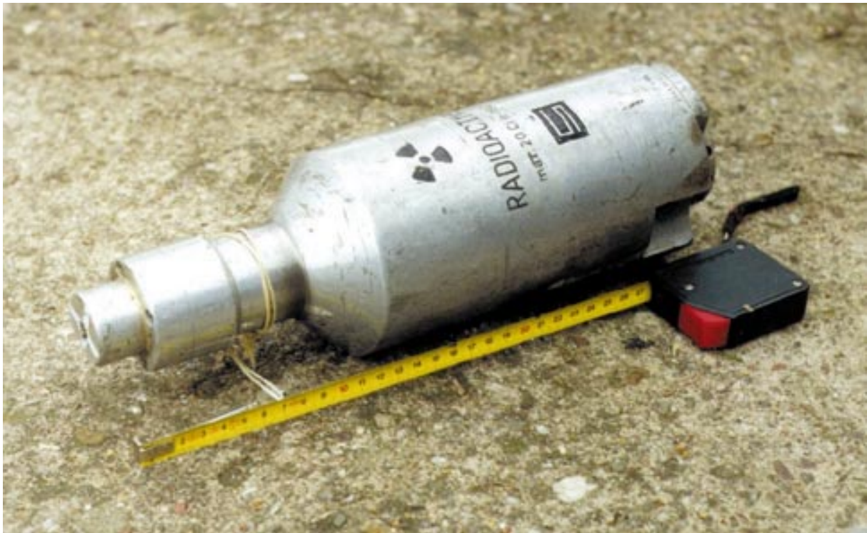
Figure 4.10 The M6 „Molch” (so-called „Little Salamander”) for weld inspections in gas line, etc. During operation, the flaw detector is placed on a remotely controlled trolley (see Fig. no. 4.12) which ensures its move in piping. This flaw detector contains ^{192}\text{Ir} source, max. 740 GBq, with uranium shield
