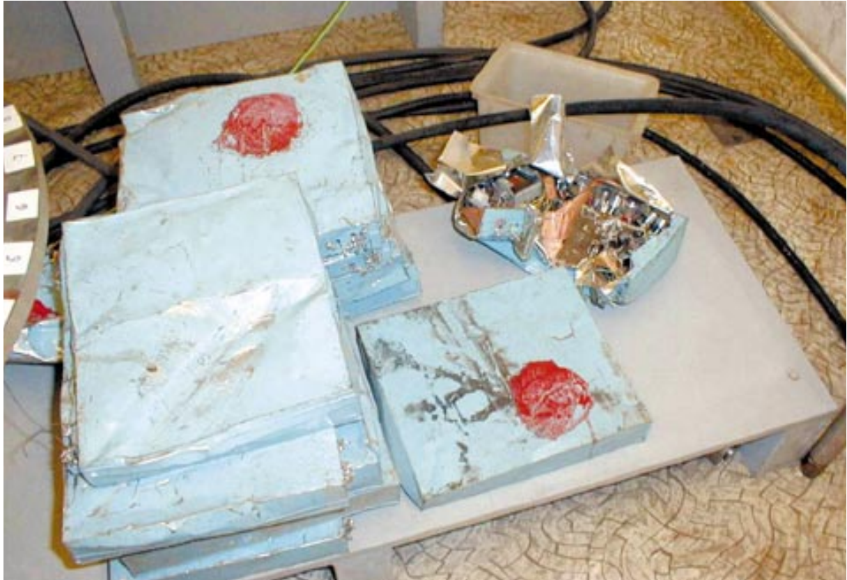
Figure 7.9 The cable amplifiers fitted with ^{226}\text{Ra} surge arresters that were found in metal scrap. Produced by Tesla Rožnov. Activity of ^{226}\text{Ra} ~ 30 kBq, dose rate in contact of 3 _Gy/hr. The photograph supplied by SÚRO
