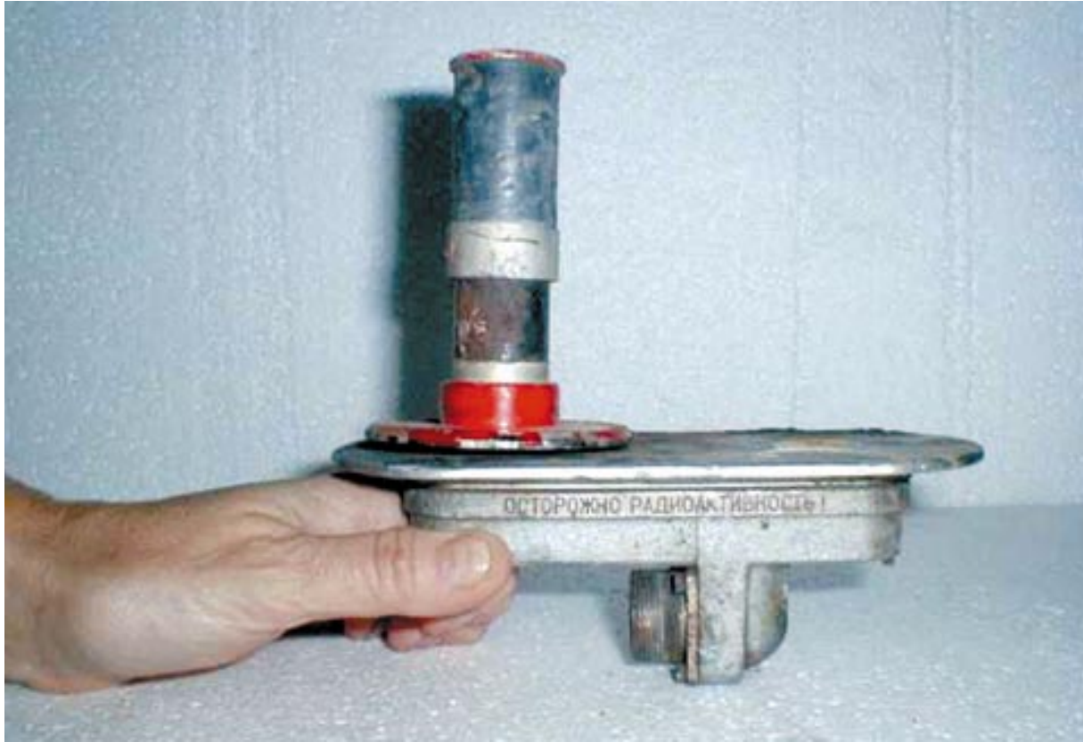
Figure 7.17 The ice thickness gauge with ^{90}\text{Sr} from the military aircrafts that was found in metal scrap. Activity up to hundreds of MBq, dose rate in contact is units of mGy/hr (no lead shield). The photograph supplied by SÚRO
