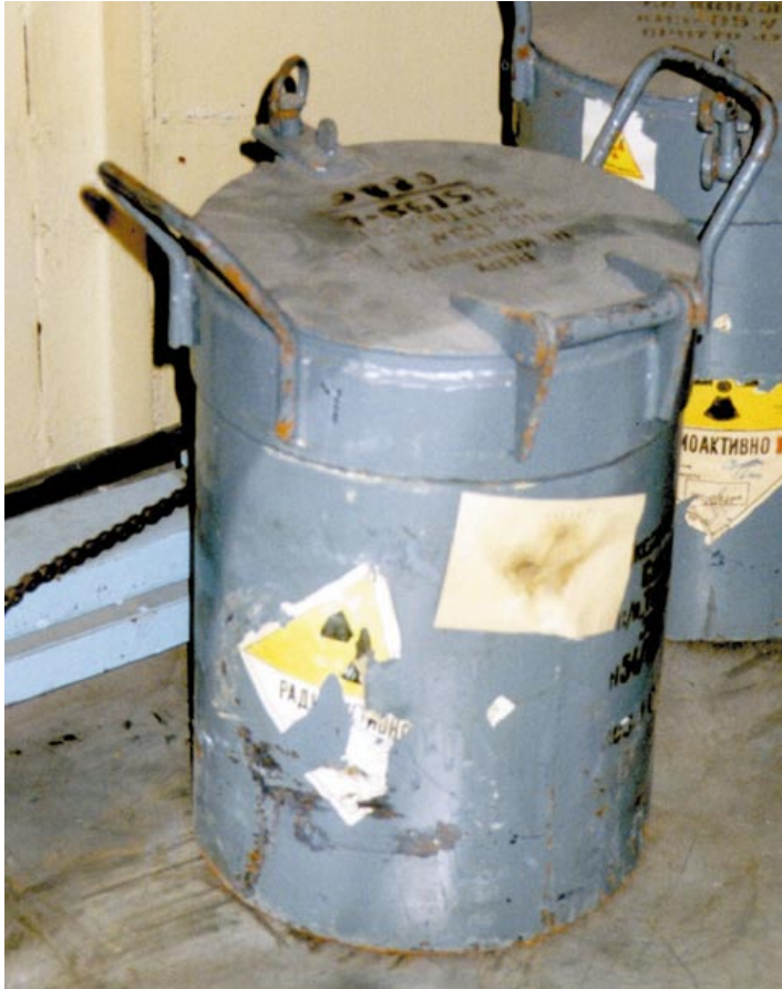
Figure 6.36 The transport vessel for the KIZ container. Made in the U.S.S.R. Dimensions of 26cm \bar{} 36cm, weight of 87 kg
