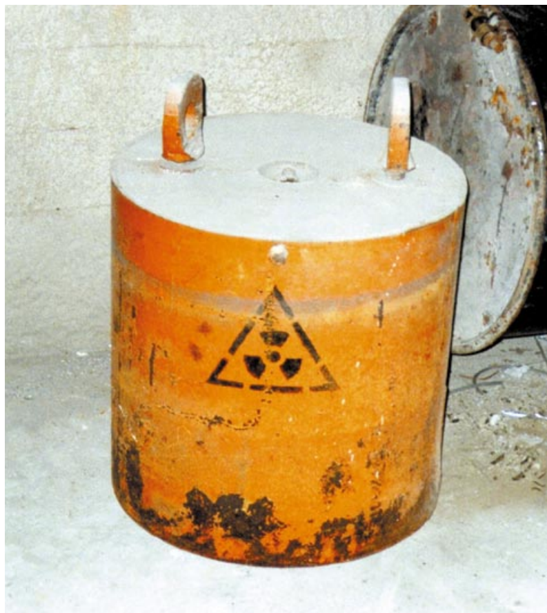
Figure 6.41 The external transport package used on waste repository. Its height is estimated to 50 – 60 cm, weight not specified
