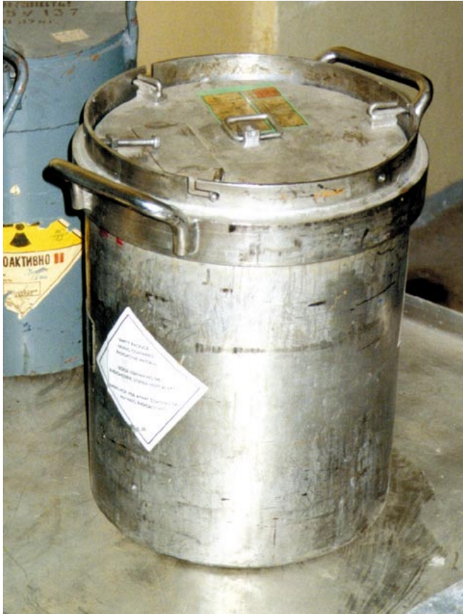
Figure 6.32 The BG-22 type container transport package, class B, produced in Germany. Dimensions 30cm \bar{} 40cm, weight including the container is 110 kg. Used for high-activity sources
