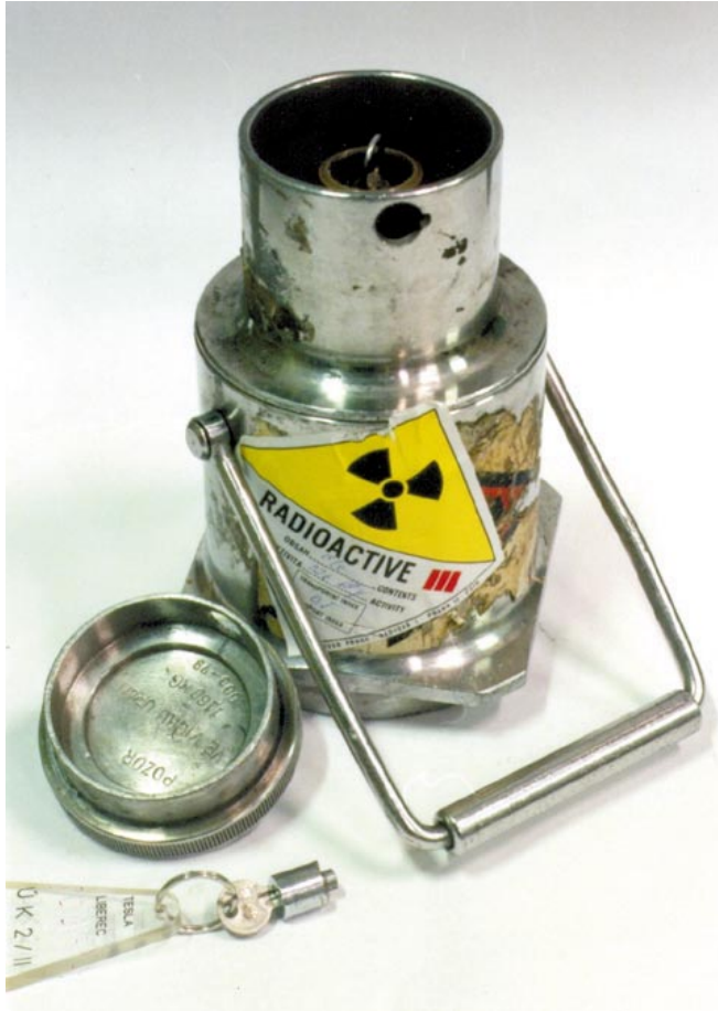
Figure 6.13 The UK 2/II transport container, class B, height of 25.5 cm, a diameter of large cylinder is 14 cm, weight of 25 kg. The container was produced in a high number of pieces and was intended for transport of max. 81 GBq of ^{137}\text{Cs} . The UK 2 and UK2/I containers were very similar
