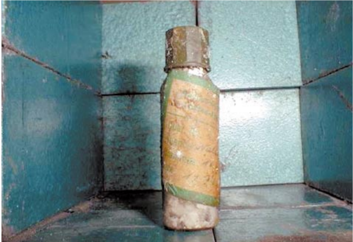
Figure 7.1 A luminescent paint with ^{226}\text{Ra} that was found in municipal waste. Produced in the 1960s, activity in order of MBq, dose rate in contact from 100 to 300 \mu\text{Gy/hr} . A possible origin in the CR: the former Mikrotechna plants. The photograph supplied by SÚRO
