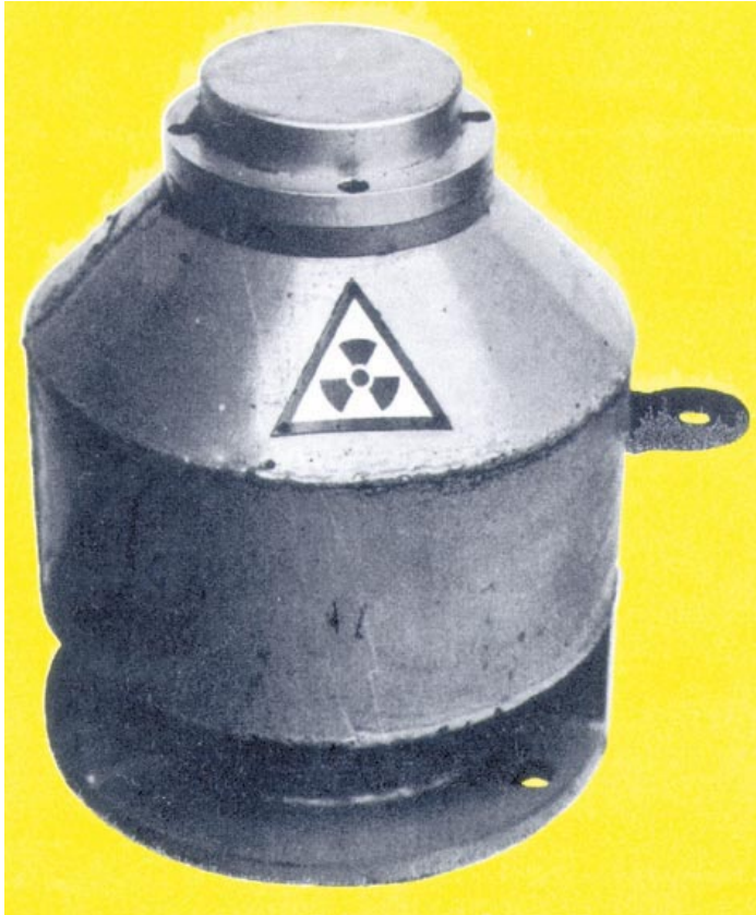
Figure 3.1 The MDG 301 level indicator shield. Its application is in reservoirs, tanks, silos, etc. It can contain either ^{60}\text{Co} with activity up to 23.3 GBq or ^{137}\text{Cs} with activity up to 116.5 GBq. The company material of the former Tesla Liberec
