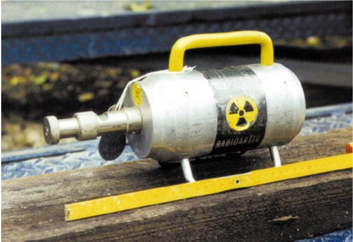
Figure 4.12 Komandogerät – the „Molch" motion controller in piping. ^{137}\text{Cs} source, max. 13 GBq. Uranium shield, the weight of the unit is 6.5 kg
