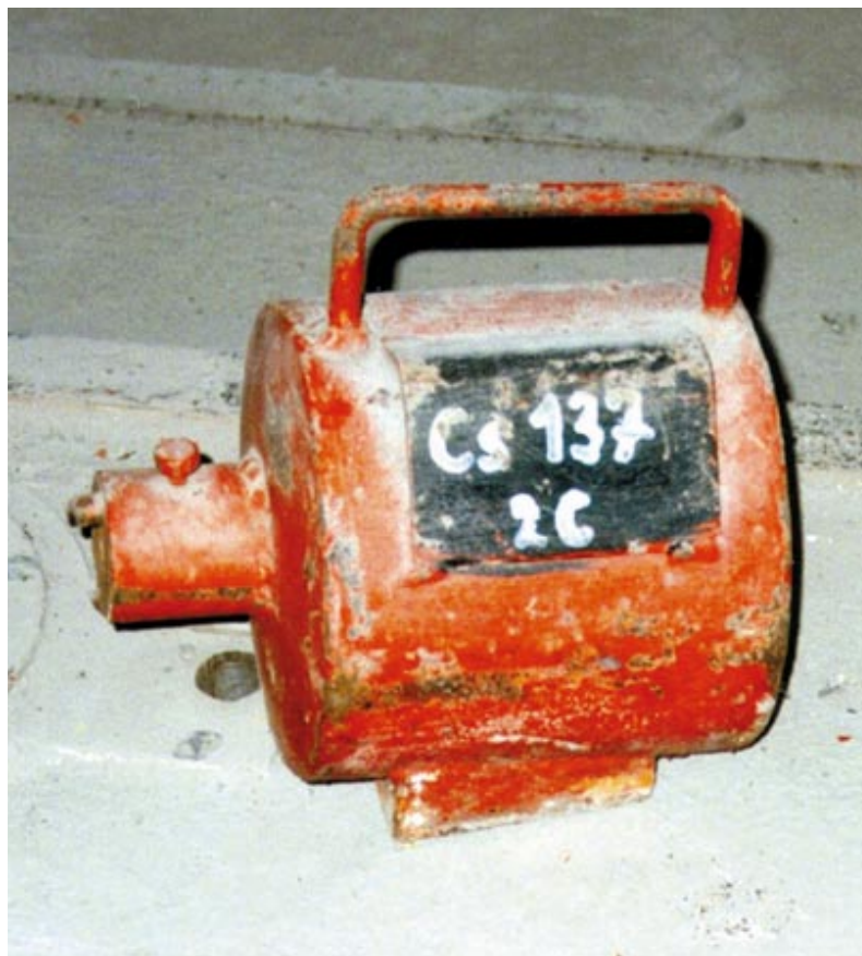
Figure 3.36 An unidentified operational container. According to the label, the ^{137}\text{Cs} source of activity of about 74 GBq was used
