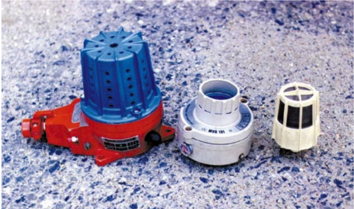
Figure 2.1 The fire detectors that were produced by the former Tesla Liberec On the left MHG 102 (2135 kBq 241Am), in the middle MHG 181 (35 kBq 241Am), on the right MHG 103 (75 kBq 241Am). The MHG 107 fire detector with 35 kBq 241Am looks like MHG 181. See also Fig. no. 2.4
