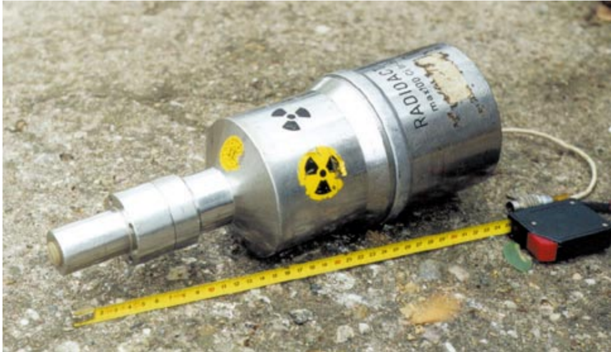
Figure 4.8 The „Molch" M18 flaw detector (so-called "Big Salamander") used for weld inspections in gas line, etc. During operation, the flaw detector is placed on a remotely controlled trolley (see Fig. no. 4.12) which ensures its move in piping. ^{192}\text{Ir} source, max. 3.7 TBq. Uranium shield
