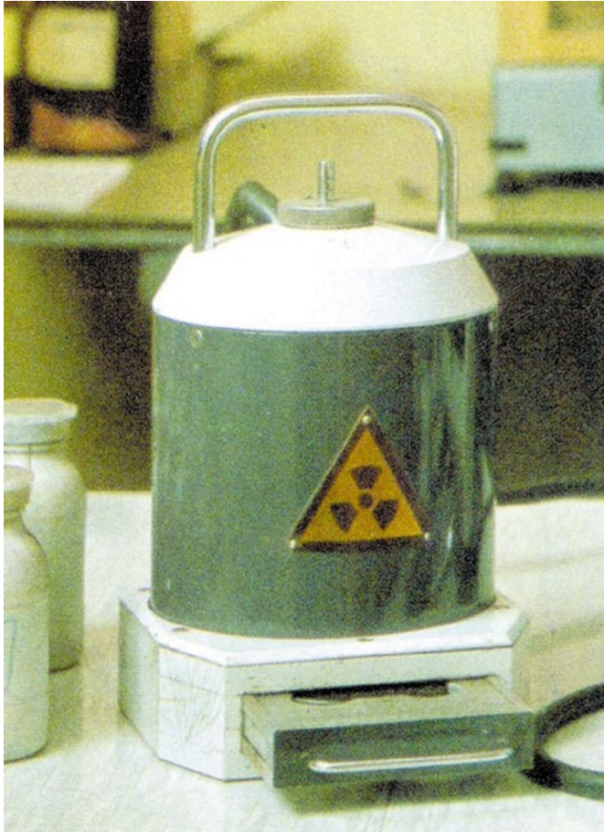
Figure 3.20 The MNG 202 laboratory ash-gauge. Dimensions of 17cm \bar{} 19cm \bar{} 28cm, weight of 8 kg. Product of the former Tesla Liberec. From the company documentation of the former Tesla Liberec
