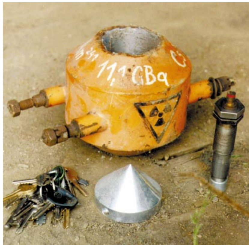
Figure 3.21 The operational container for the ash-gauge of domestic production, however very often used in the other equipment. Size of 20 cm, weight of 25 kg
