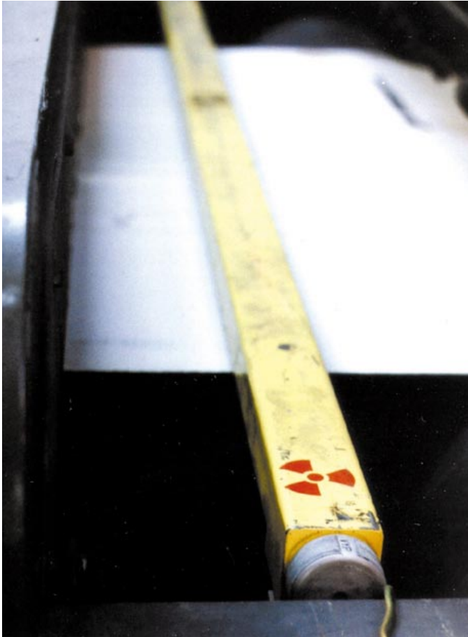
Figure 1.5 The detail of the electrostatic charge eliminator
