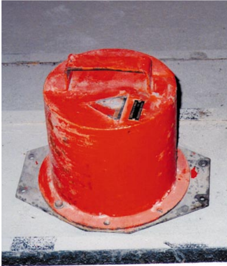
Figure 3.14 The protective collimator shield with MDN 202 source for density measurements. The cylinder is available in the dimensions of 23cm \times 21cm, weight of 22 kg. Product of the former Tesla Liberec, ČSSR
