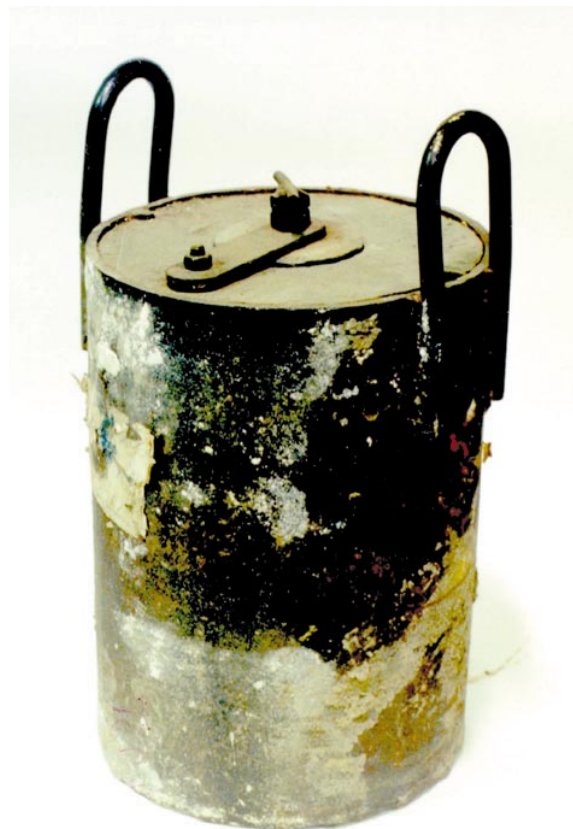
Figure 6.37 The older KIZ transport container, made in the U.S.S.R., now without identification. Steel package, lead shield, cylinder dimensions of 22cm \bar{} 30cm, weight of about 100 kg
