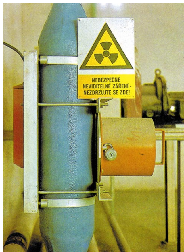
Figure 3.15 The collimator arrangement with MDN 202 source (see the previous figure). The collimator and the source are positioned below the orange cover on the right, the probe is on the left. Liquids or loose substances being measured flow through the piping. From the company documentation of the former Tesla Liberec
