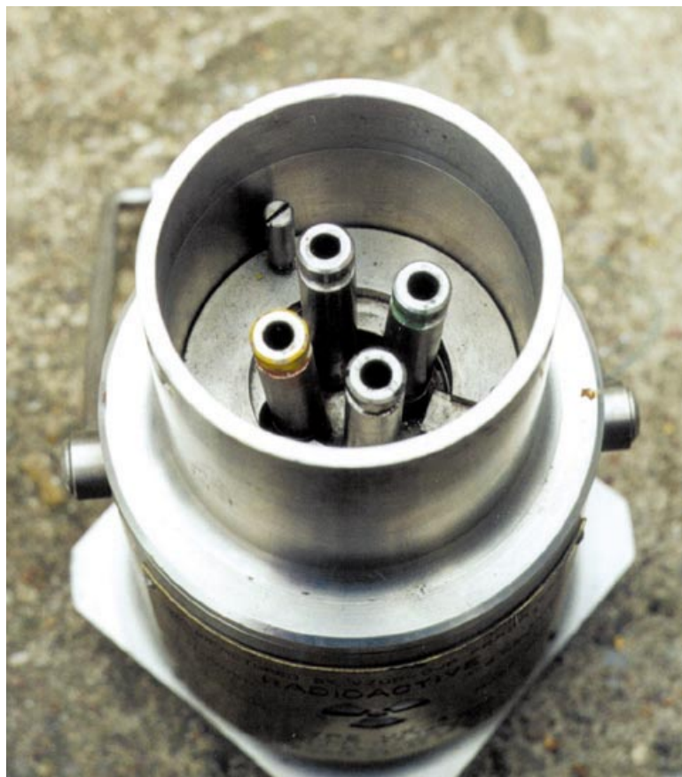
Figure 6.16 The UK-4 transport container is fitted with four cavity closures with a diameter of 7.5 mm and a length of 137 mm
