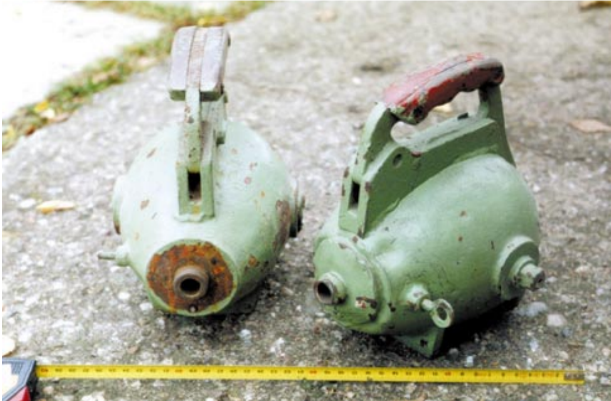
Figure 4.19 The transport and operational containers for the flaw detector sources dated from the 1950s and the 1960s. The source of ^{137}\text{Cs} , and the maximum activity of about 37 GBq was used at that time. There is a channel in the „egg-shaped“ container from which the source is ejected to the operational position by means of a bar. Lead shield and steel jacket. Its weight is about 22 kg
