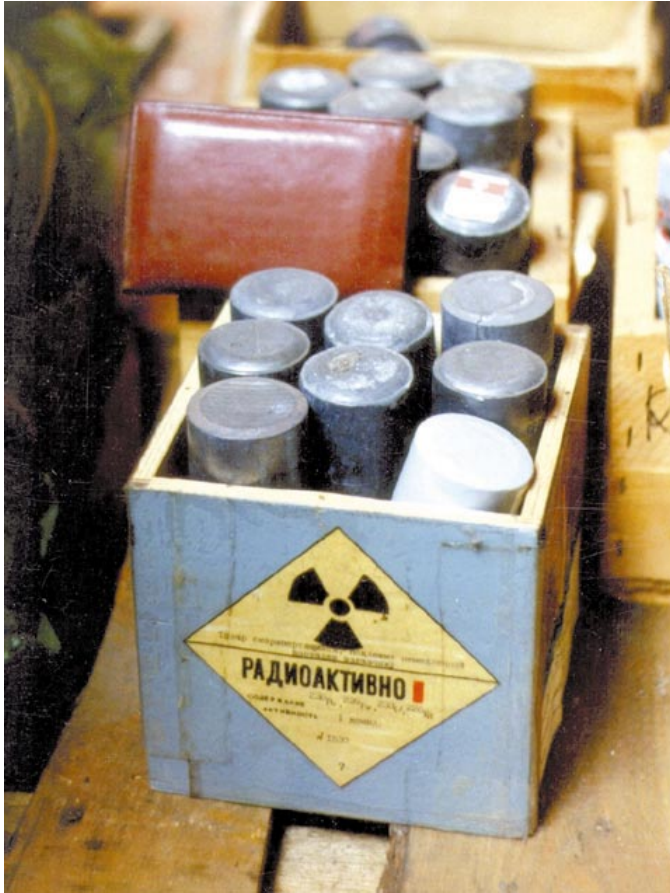
Figure 6.48 The external small lead containers for the sources of activities up to hundreds of kBq
