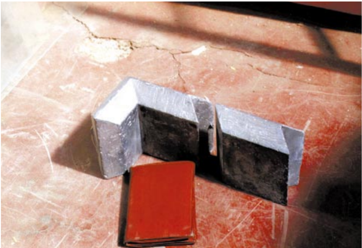
Figure 1.6 Lead shielding blocks
