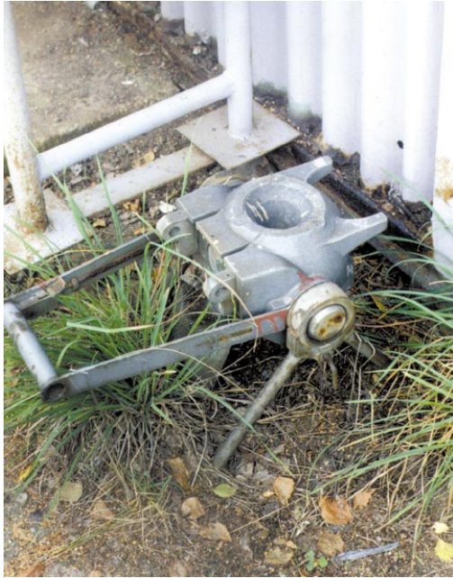
Figure 4.21 A fragment of the operational container used for the flaw detector source that was ejected from the central channel by means of a bar. Produced by VEB Transformatoren - u. Röntgenwerk Dresden, East Germany. Lead shield and probably cast iron jacket. Used for ^{137}\text{Cs} . Its weight with the stand was about 55 kg
