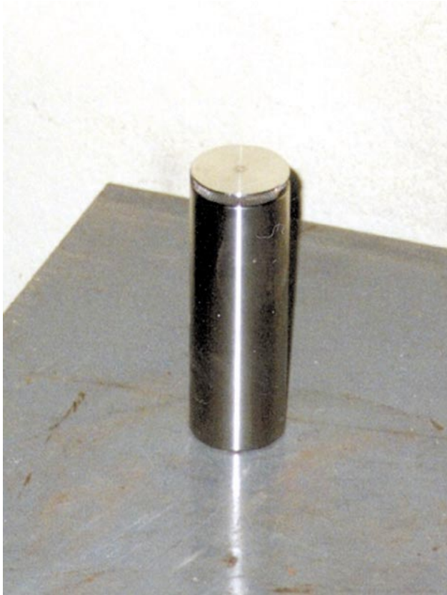
Figure 6.42 The cavity closure. Dimensions of 4cm \bar{} 11cm, weight of 250 g
