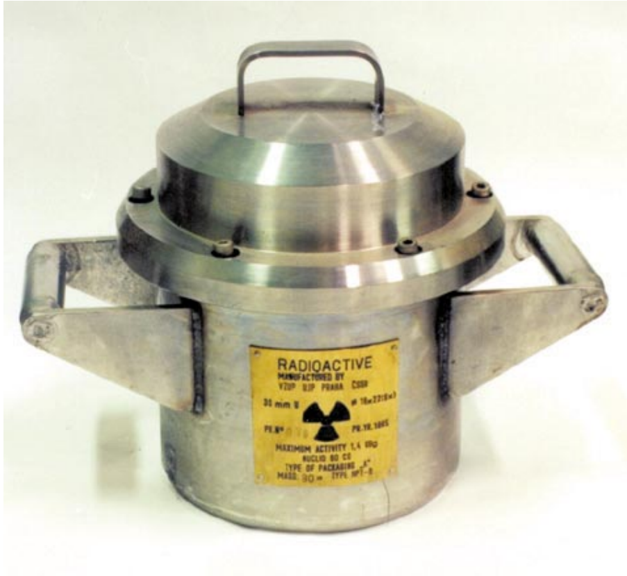
Figure 6.28 The HPT-6 transport container, class A, uranium shield, diameter of 25 cm, height of 27 cm, weight of 80 kg. Intended for transport of the maximum 1.4 GBq of ^{60}\text{Co} , but also for ^{137}\text{Cs} and the other nuclides
