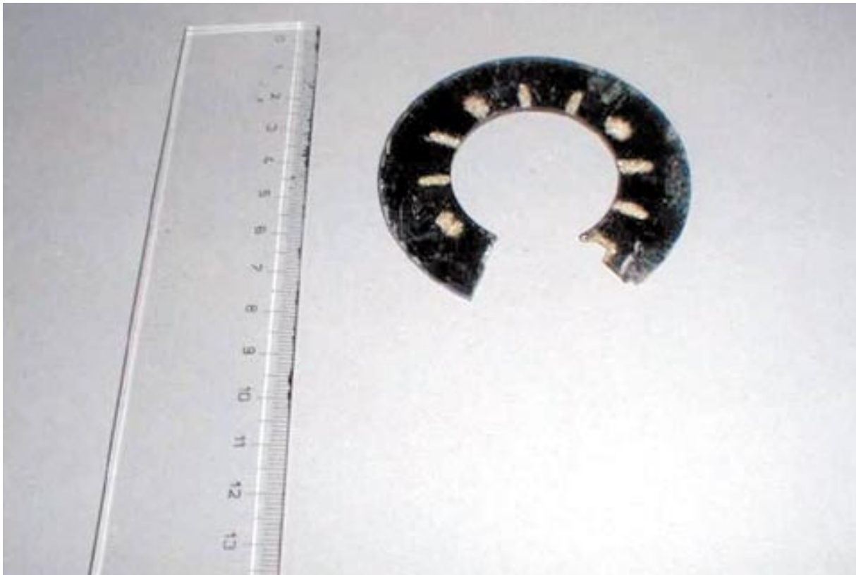
Figure 7.4 The matrix of clock dials coated with a ^{226}\text{Ra} and ^{90}\text{Sr} luminescent paint and found in municipal waste. The photograph supplied by SÚRO
