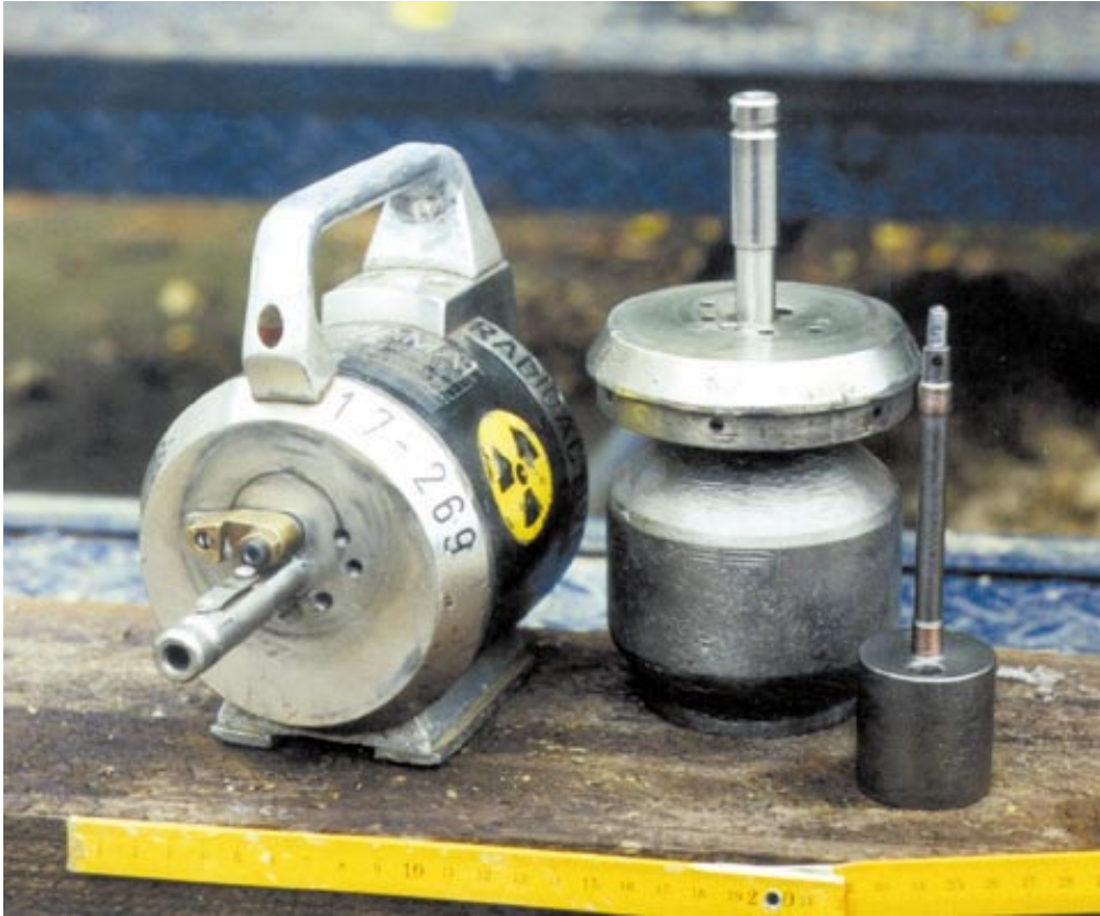
Figure 4.14 A dismantled Gammamat TIF. On the right: two separated parts of the depleted uranium shield. The unit can contain max. 3.75 TBq of ^{192}\text{Ir}
