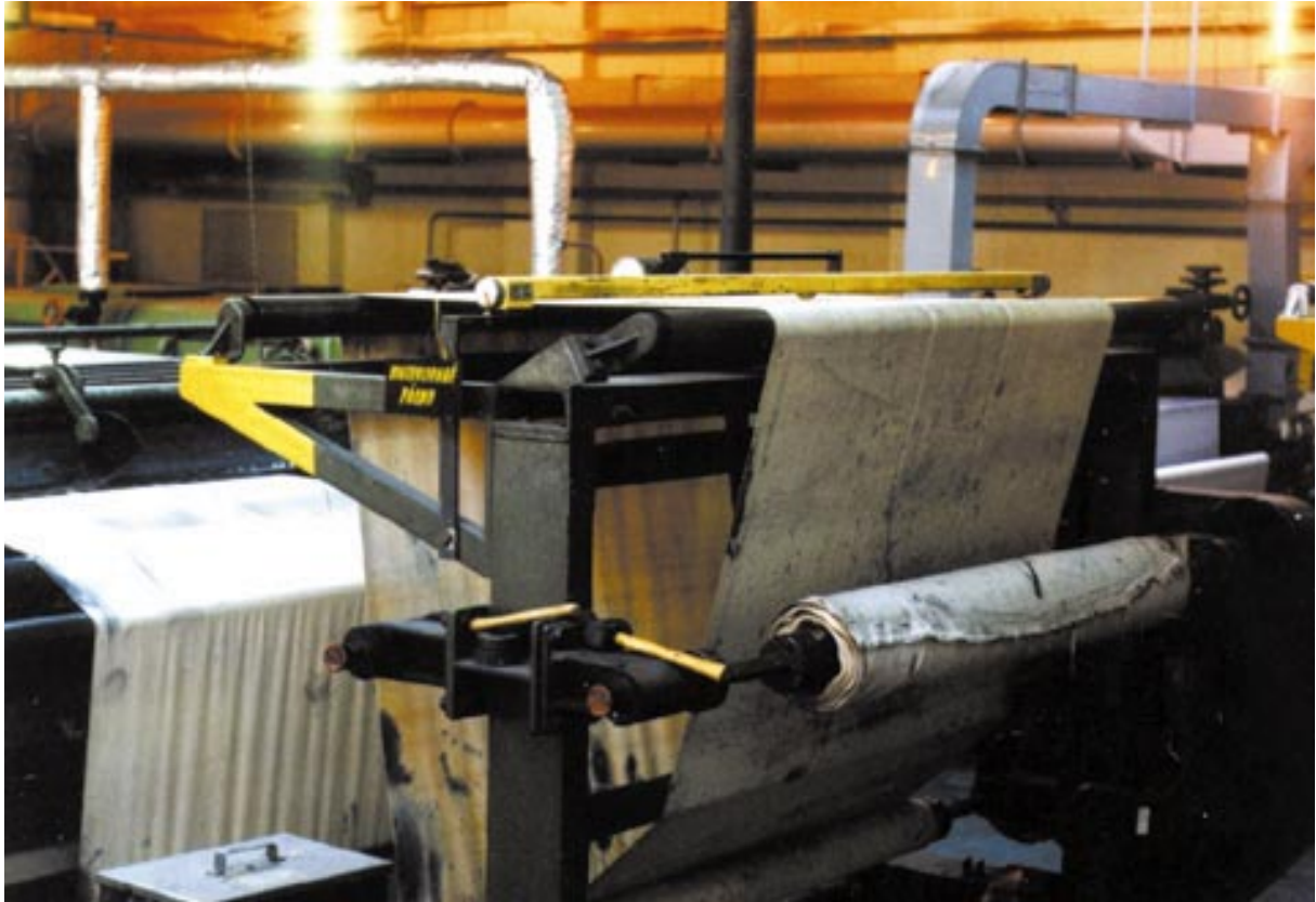
Figure 1.3 The electrostatic charge eliminator (the yellow bar above) on a rubber coating machine. The high-intensity alpha radiation eliminates electrostatic charge on the surface and it also reduces the danger of explosion due to thinner vapour
