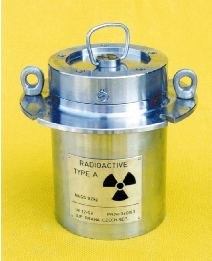
Figure 6.11 The UK-12-SV type transport container, class A. Uranium shield, weight of 92 kg (for UK-12-S only 84 kg). Produced by ÚJP Praha. The photograph from ŠKODA – ÚJP Praha, a.s.
