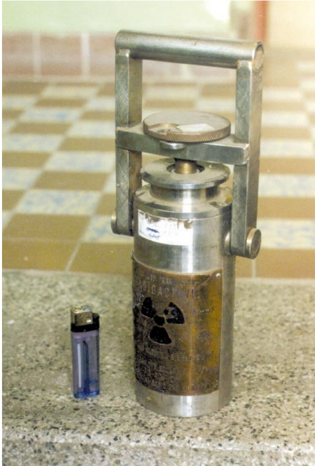
Figure 6.9 The older TO-ACs-21 transport container, A type. Uranium shield, total height of 30 cm, weight of 15 kg, max. 5 \pm 0.7 GBq of ^{137}\text{Cs}
