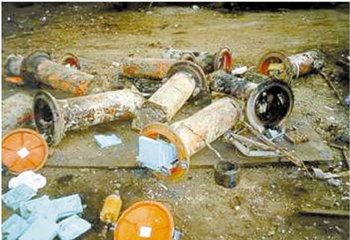
Figure 7.10 The cable amplifiers that are fitted with ^{226}\text{Ra} surge arresters. A general view on the complete system. The photograph supplied by SÚRO
