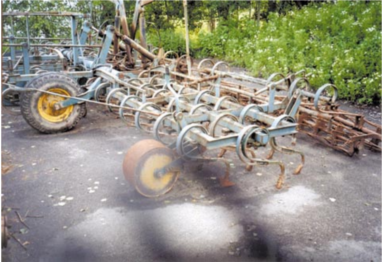
Figure 7.13 The agricultural machine (i.e. cultivator), some of its elastic blade holders were produced in ^{60}\text{Co} contaminated heat. The photograph supplied by SÚJB
