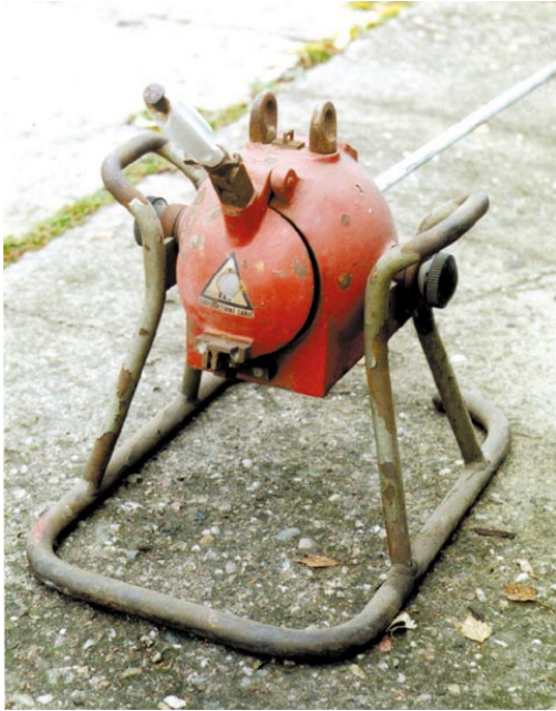
Figure 4.16 The OK 0.5 type flaw detector dated from 1962. The operational shield is swinging, ^{137}\text{Cs} source is ejected on a bar from behind. Produced by: První brněnská strojírna, Z.K.G. The weight with the stand is about 55 kg
