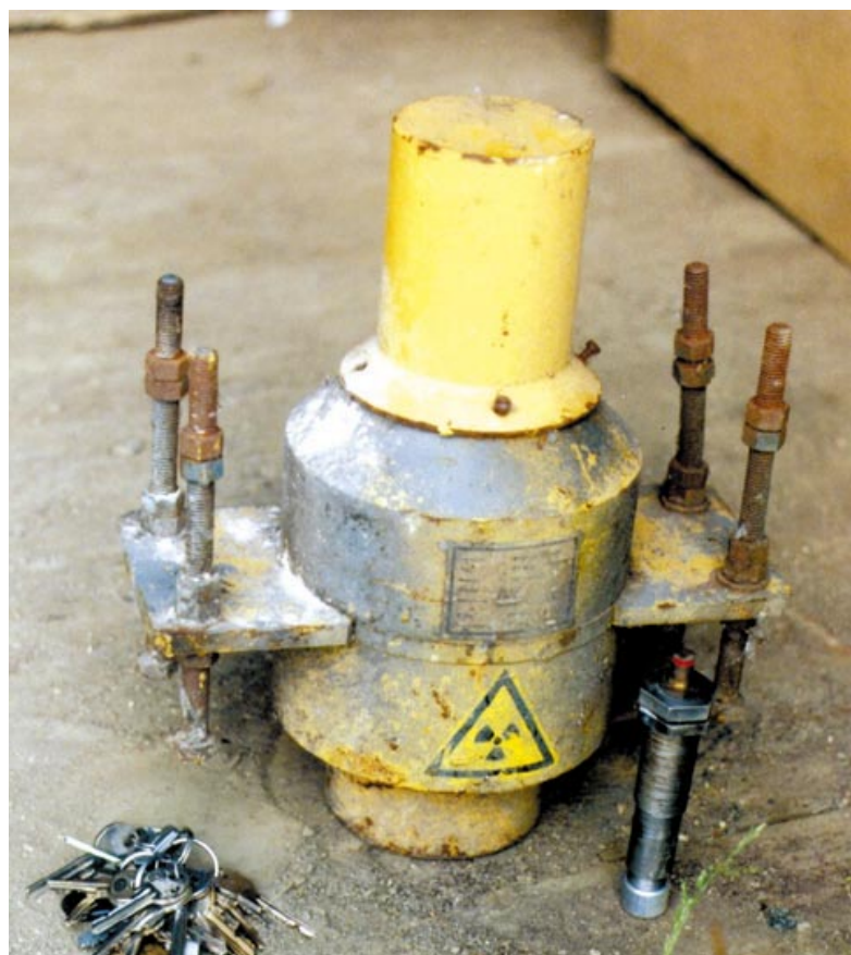
Figure 3.23 The operational container for the ash-gauge produced in the former East Germany. The container with a conical shield - the source is in the non-operating state. On the right, the screw fitted with a source and which is unscrewed from a shield
