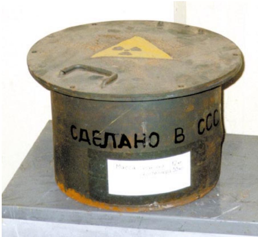
Figure 6.38 A fragment of the Soviet transport cask used for a container. The weight of cask (12 kg) and the container (55 kg) is indicated on the label
