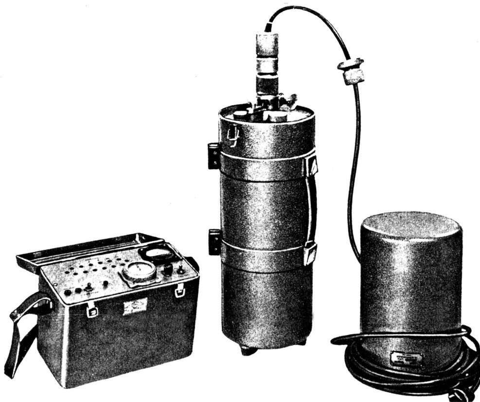
Figure 3.27 The old Soviet GGP-1 type radiation logging hydrometer for shallow bores. The source is ^{137}\text{Cs} . The dimensions of the probe are 5cm \bar{\imath} 50cm and its weight is 3 kg. The photograph from the catalogue: Izdělja jadernogo priborostrojenja stran-členov SEV
