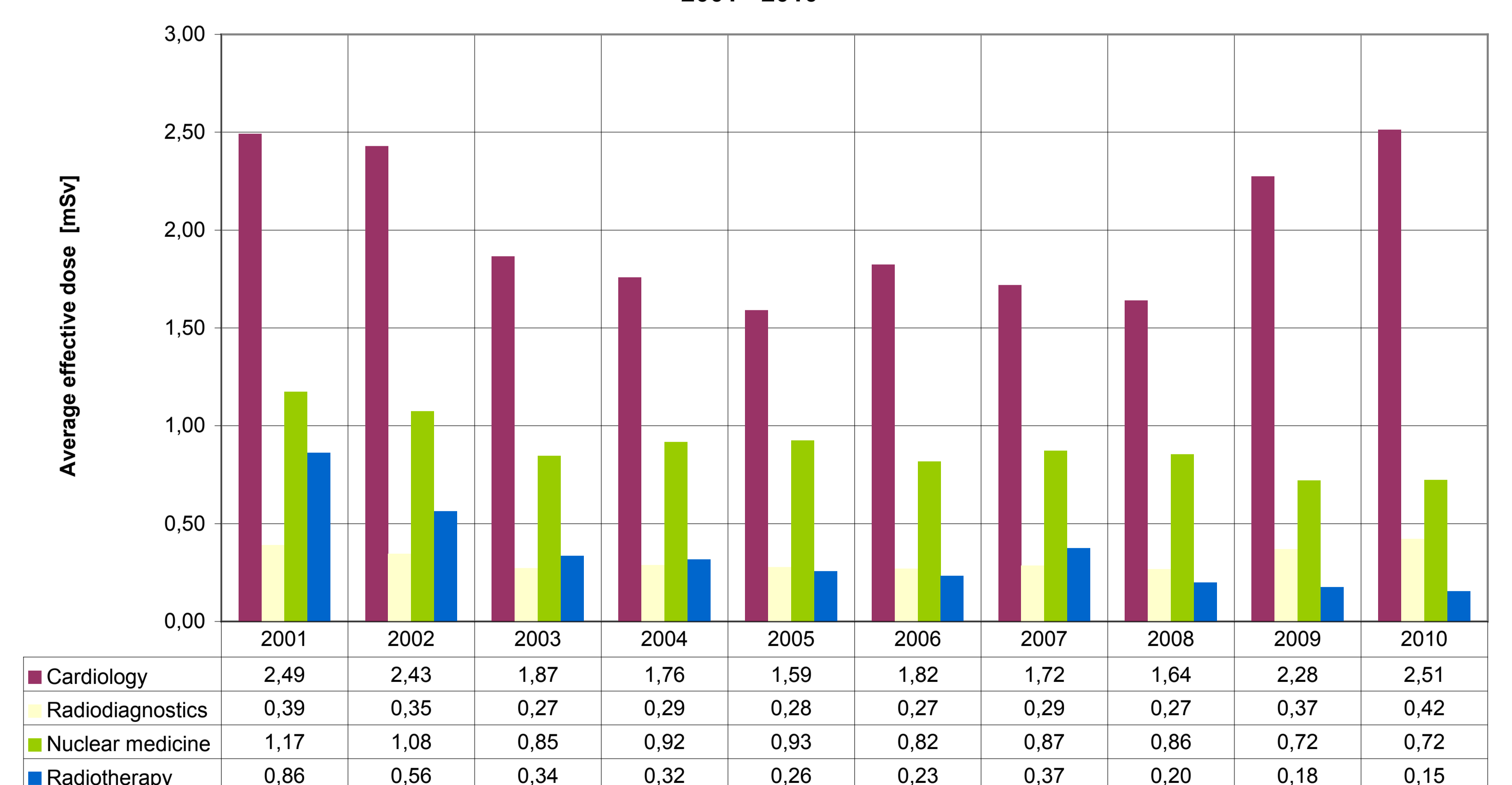
Fig. 6: Average effective dose of radiation workers in various professional groups in years 2001 - 2010
